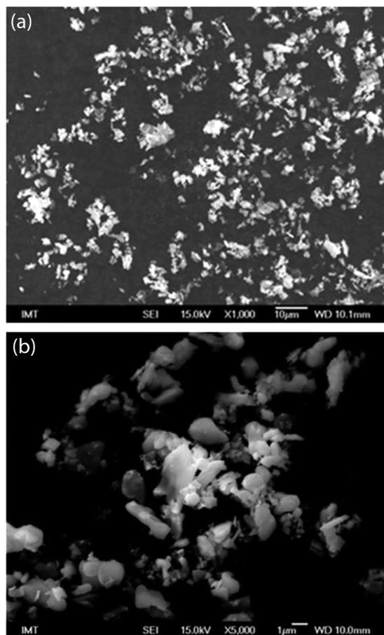
**Figure 1:** SEM image of  $\text{Al}_2\text{O}_3$  ultrafine particles at various magnifications
