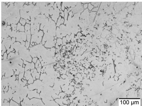
**Figure 3:** Cast microstructure of austenitic stainless steel with 6 % of  $\delta$ -ferrite and  $\text{Al}_2\text{O}_3$  ultrafine particles
