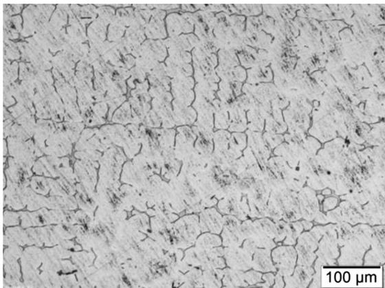
**Figure 2:** Cast microstructure of austenitic stainless steel with 6 % of  $\delta$ -ferrite
