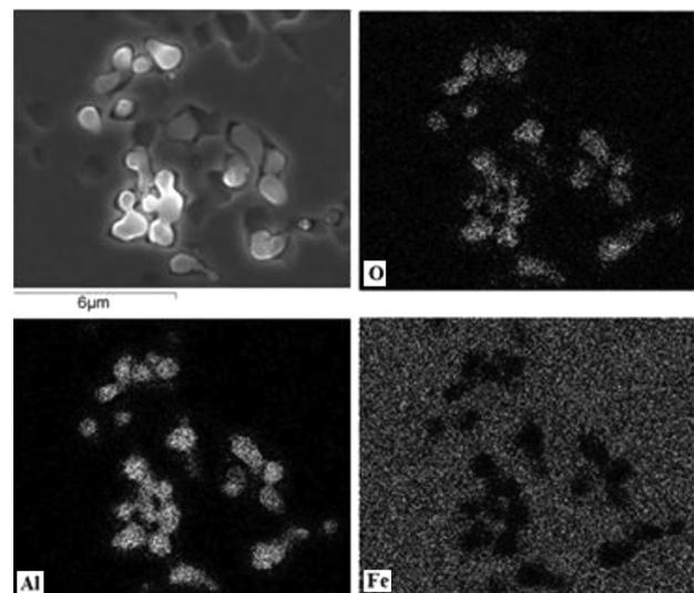
**Figure 5:** SEM elemental analysis of  $\text{Al}_2\text{O}_3$  ultrafine particles in the cast microstructure of austenitic stainless steel
