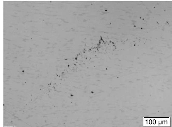
**Figure 4:** Cast microstructure of austenitic stainless steel with  $\text{Al}_2\text{O}_3$  ultrafine particles inserted into the melt (experiment 2)
