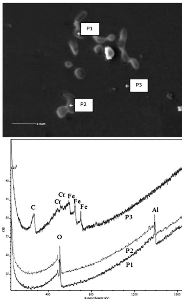
**Figure 6:** AES spectrum of the  $\text{Al}_2\text{O}_3$  ultrafine particles in the cast microstructure of austenitic stainless steel
