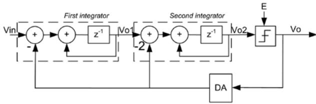
Fig. 3: 2<sup>nd</sup> order sigma-delta modulator
