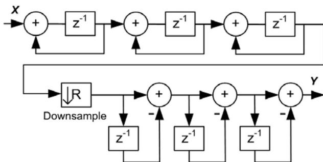
Fig. 4: Decimation using 3<sup>rd</sup> order CIC filter
