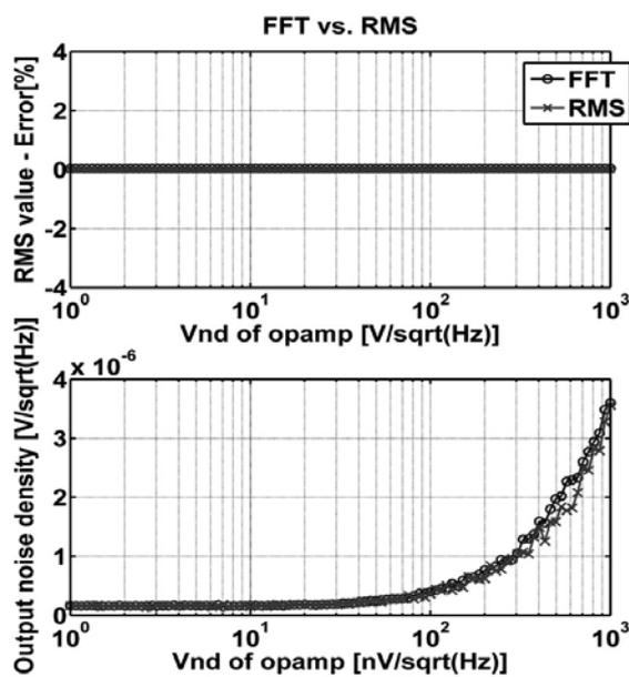
Fig. 12: RMS error and standard deviation of RMS as a function of input noise voltage of the first amplifier of the modulator (o : FFT results, x: RMS results )
