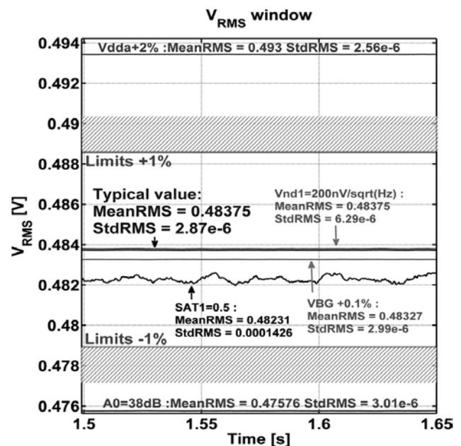
Fig. 13: RMS voltage from system level simulations at different parameters
