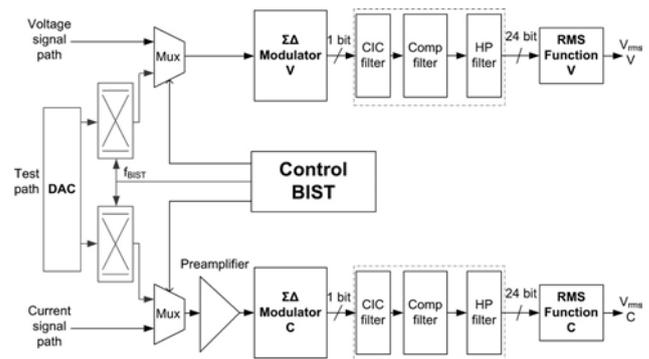
Fig. 1: Block diagram of energy meter ASIC
