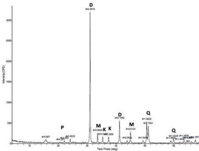
Figure 4: XRD diffractogram pattern of Alaguntan marble (Sample 2).
