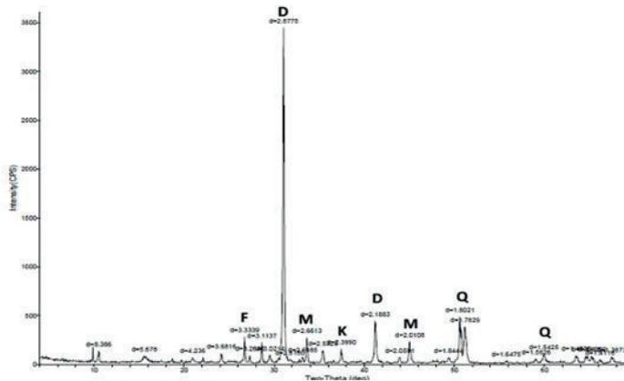
Figure 3: XRD diffractometer pattern of Alaguntan marble (Sample 1).
