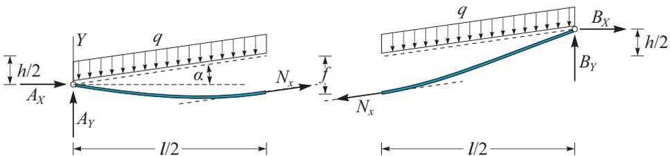
$$\begin{aligned} \sum_{\text{levi}} M^A = 0 &\rightarrow N_x \left( f - \frac{h}{2} \right) \cos \alpha + N_x \frac{l}{2} \sin \alpha - q \frac{l}{2} \frac{l}{4} = 0 \rightarrow \\ &\rightarrow N_x = \frac{q l^2}{8} \frac{1}{\left( f - \frac{h}{2} \right) \cos \alpha + \frac{l}{2} \sin \alpha} = 6281 \text{ kN}, \end{aligned}$$
