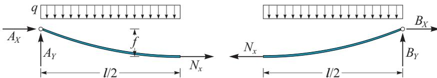
$$\sum_{\text{levi}} M^A = 0 \rightarrow N_x f - q \frac{l}{2} \frac{l}{4} = 0 \rightarrow N_x = \frac{q l^2}{8 f} = 6250 \text{ kN},$$
