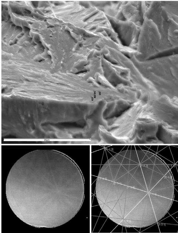
**Figure 17:** (a) SE micrograph of the fracture surface of the steel quenched from 1250 °C in water at 70 °C and reheated at 750 °C; (b) EBSD analysis and indexing of a cleavage facet <sup>23</sup>
