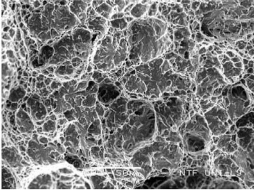
**Figure 12:** As delivered steel, fracture surface at 22 °C
