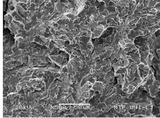
**Figure 15:** Steel quenched in water from 920 °C and fractured at -60 °C
