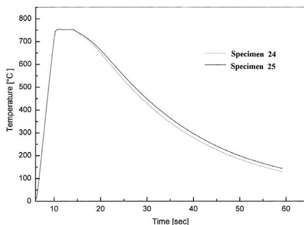
Figure 1: Reheating cycle for specimens
