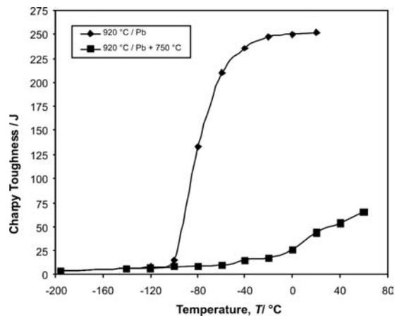
**Figure 9:** Dependence Charpy toughness versus testing temperature after cooling from 920 °C in lead bath at 400 °C and after reheating at 750 °C
