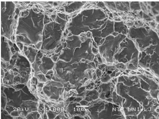
**Figure 14:** Steel quenched from 920 °C in water and fractured at 0 °C
