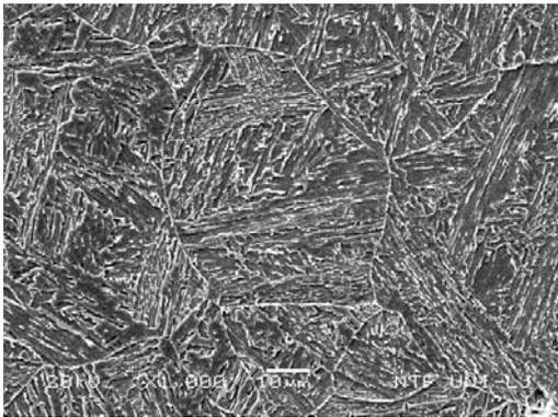
**Figure 5:** Microstructure after lead bath quenching from 1250 °C
