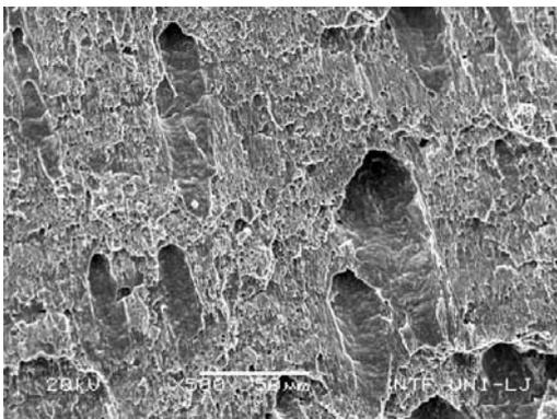
**Figure 13:** As delivered steel, fracture surface at 22 °C. Shear decohesion
