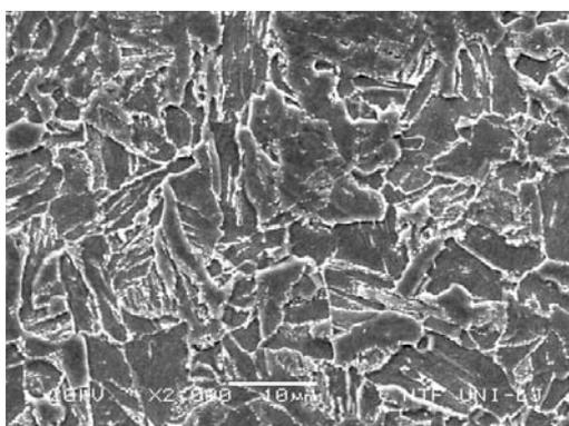
**Figure 2:** Microstructure of as delivered steel
