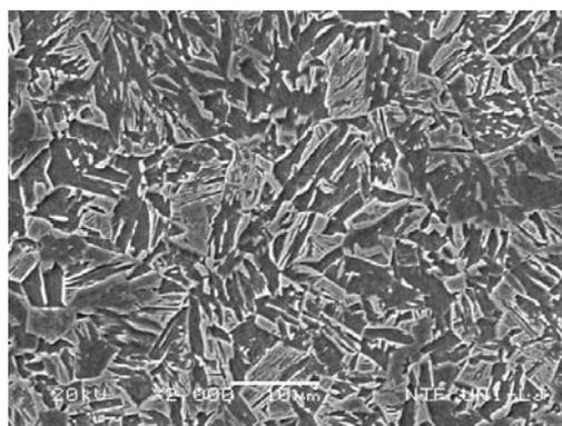
**Figure 3:** Microstructure after water quenching from 920 °C
