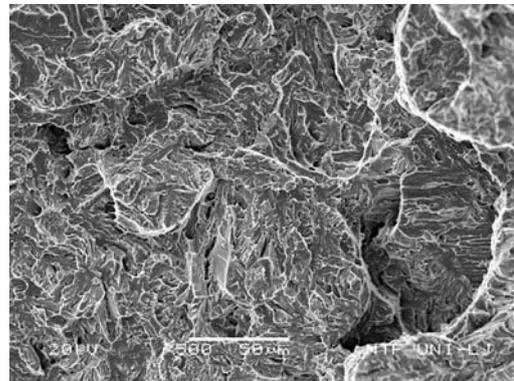
**Figure 16:** Steel quenched from 1250 °C in lead and fractured at -60 °C
