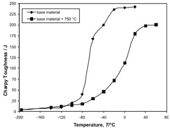
**Figure 7:** Dependence Charpy toughness versus testing temperature for the steel with the as delivered steel and after reheating at 750 °C
