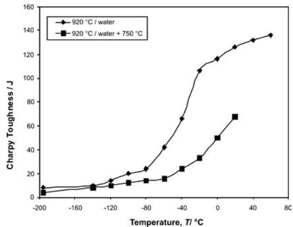
**Figure 8:** Dependence Charpy toughness versus testing temperature after hot water quenching from 920 °C and after reheating at 750 °C
