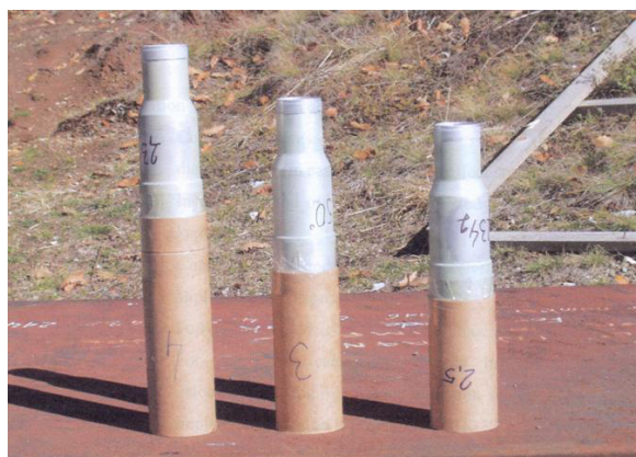
Fig. 10. Three typical shaped charges with different standoff distances
