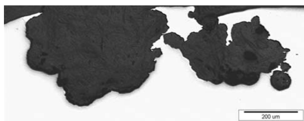
Figure 5: Micrograph of cross-section of the corrosion pit on the bent edge. Local corrosion advanced deep into the material of the case wall
