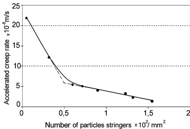
**Figure 1:** Dependence of accelerated creep rate on the number of stringers of carbide particles in martensite in 0.18C11.5Cr1.08 Mo0.29V steel.<sup>36</sup>
