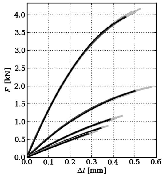
**Figure 6:** Force-displacement diagrams for 15° to 90° specimens (black – identified, grey – experiments)
