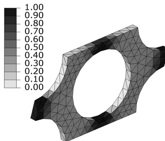
Figure 10: Distribution of damage factor (factor is not calculated for fibers, deformation is magnified 10 times)
