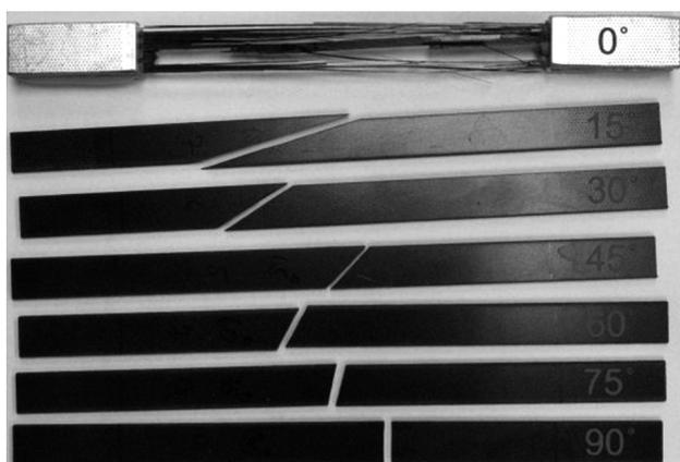
Figure 2: Cracked specimens with aluminum tabs on a specimen with a 0° orientation<sup>2</sup>
