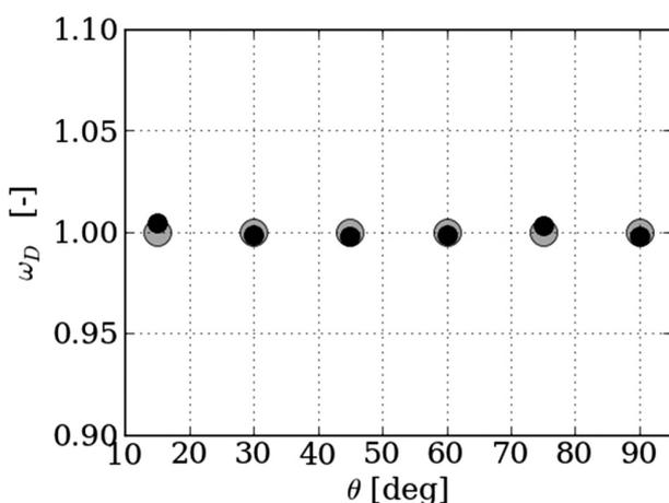
Figure 8: Maximum damage factors for specimens from 15° to 90° (black – identified, grey – experiments)
