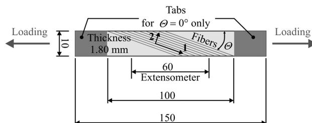
Figure 1: Geometry of composite coupons (mm)<sup>2</sup>
