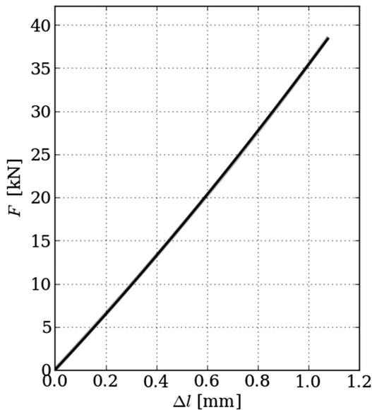
**Figure 5:** Force-displacement diagram for 0° specimen (black – identified, grey – experiments)
