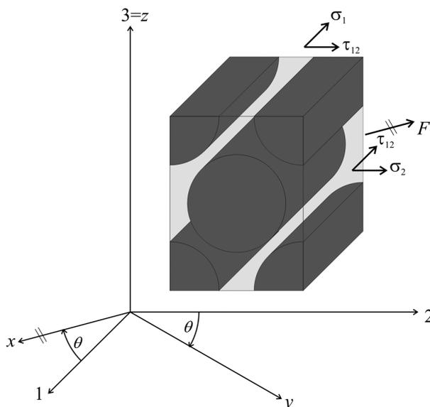
Figure 4: Rotated coordinate systems and loading of the unit cell
