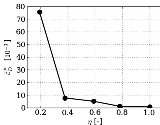
Figure 9: Dependency of the equivalent plastic strain at the onset of damage on the triaxiality stress factor
