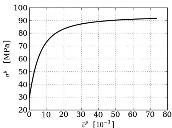
Figure 7: Work-hardening curve
