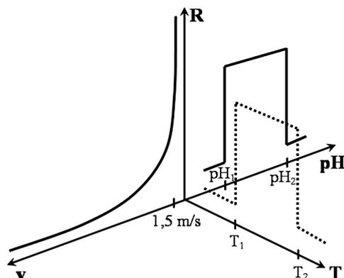
**Figure 2:** Schematic relationship between the flow velocity and the pH of water and the temperature *T* with respect to the corrosion rate *R*
