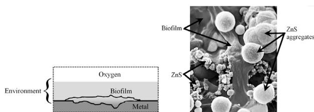
**Figure 1:** Components of the environment for the development of MIC (right) and microscopic photograph of biofilm in the case of zinc corrosion (left) <sup>3</sup>
