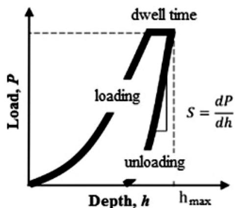
**Figure 2:** Load,  $P$ , against depth,  $h$ , during the nanoindentation test
