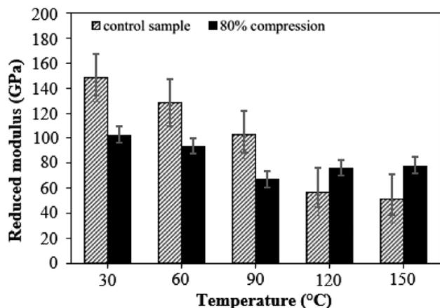
**Figure 7:** Reduced modulus against temperature for the Sn-0.7Cu alloy at different conditions
