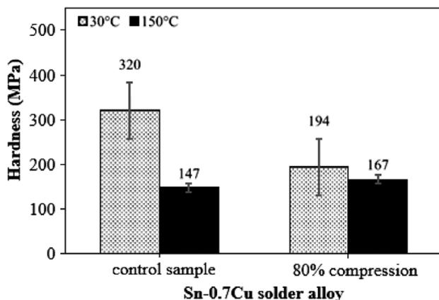
**Figure 5:** Comparison of the hardness values for Sn-0.7Cu solder-alloy samples treated at 30 °C and 150 °C
