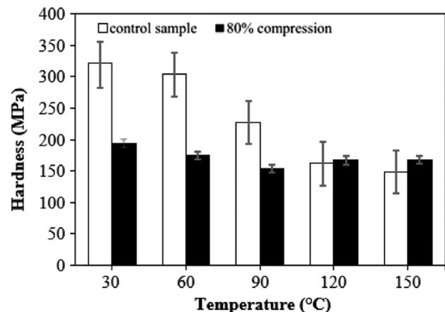
Figure 4: Hardness versus temperature for the control and thermomechanically treated solder-alloy samples
