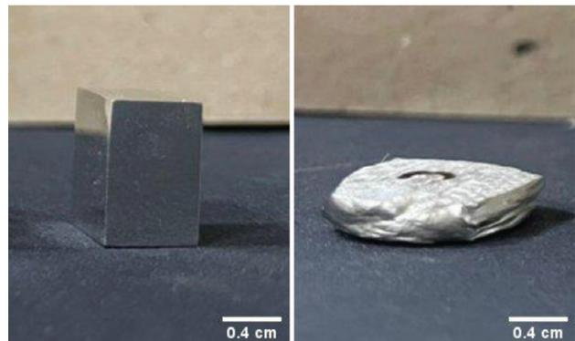
**Figure 1:** Sn-0.7Cu solder alloy before (left) and after compression (right)
