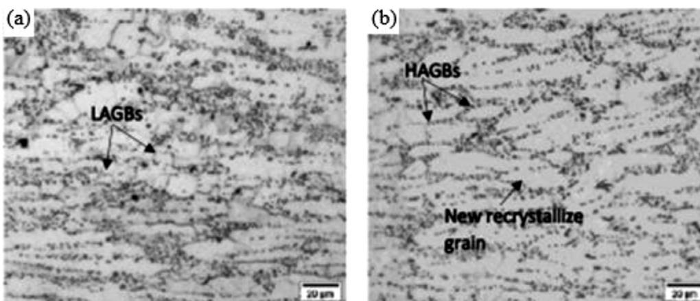
**Figure 9:** IFM images of Sn-0.7Cu after thermomechanical treatment at: a) 30 °C, b) 120 °C
