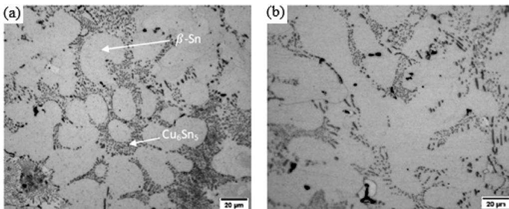
**Figure 8:** IFM images of Sn-0.7Cu after heat treatment at: a) 30 °C, b) 120 °C
