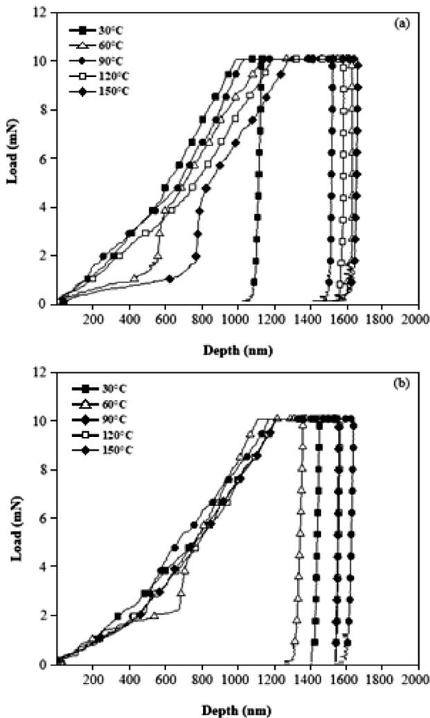
Figure 3: Load-depth graphs of Sn-0.7Cu solder alloy after: a) heat treatment, b) thermomechanical treatment
