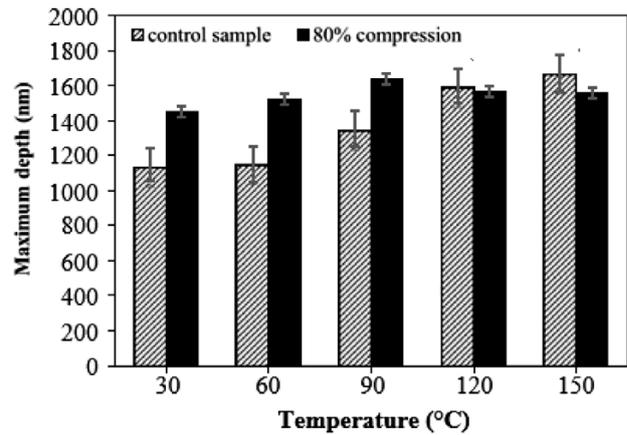
**Figure 6:** Maximum depth for the Sn-0.7Cu solder-alloy sample after heat treatment and thermomechanical treatment
