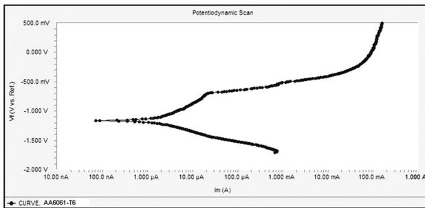
Figure 12: Polarization curves of the AA6061-T<sub>6</sub> parent metal
