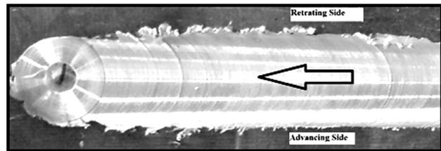
Figure 6: Friction-stir welded joint of AA6061-T<sub>6</sub>
