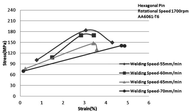
Figure 5: Engineering stress-strain curves for AA6061-T<sub>6</sub> with a hexagonal pin
