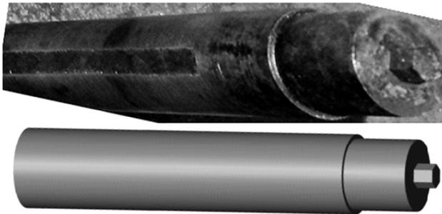
**Figure 3:** Geometry of the hexagonal tool-pin profile used in the present study**Slika 3:** Geometrija šestokotne konice, uporabljene pri preiskavah
