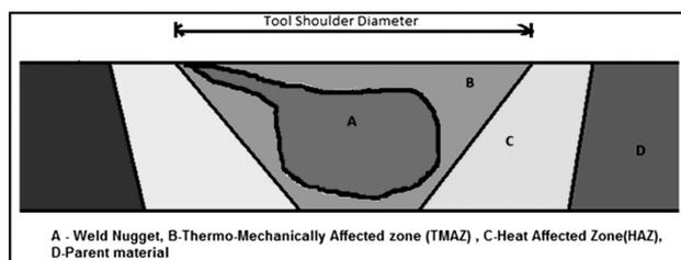
Figure 2: Different regions of a FSW joint
