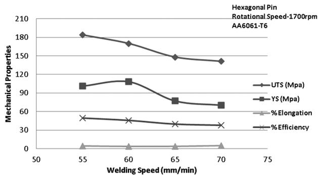
Figure 4: Effect of the welding speed on the mechanical properties of AA6061-T<sub>6</sub>
