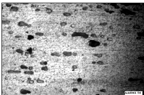
**Figure 8:** Optical micrograph of the AA6061 parent metal
