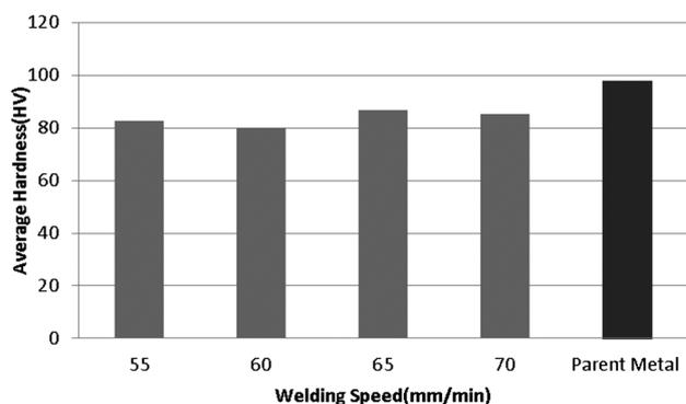
Figure 7: Effect of the welding speed on the microhardness of AA6061-T<sub>6</sub>
