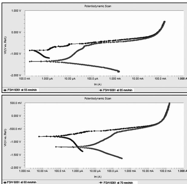
Figure 13: Polarization curves of AA6061 at the welding speeds of 55–70 mm/min
