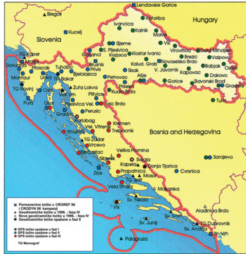
Figure 4: CROREF'96/CRODYN'96 GPS measuring campaigns (Bašić et al., 2000).
