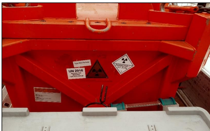
Figure 20: Outgoing shipment of ^{137}\text{Cs} in a type B(U) package, accomplished in 2023
