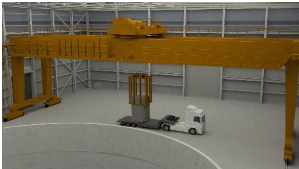
Figure 18: An N2d container being unloaded from a transport vehicle by a gantry crane and a special gripper
