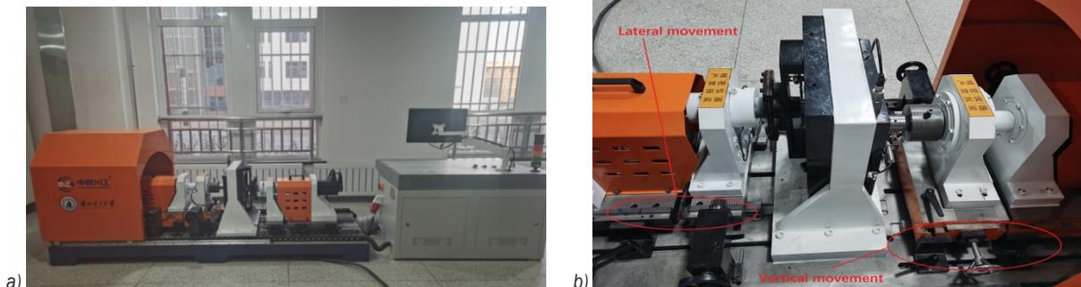
**Fig. 5.** The elliptic gear transmission test; a) overall view of the test bench, and b) partial view of the test bench
