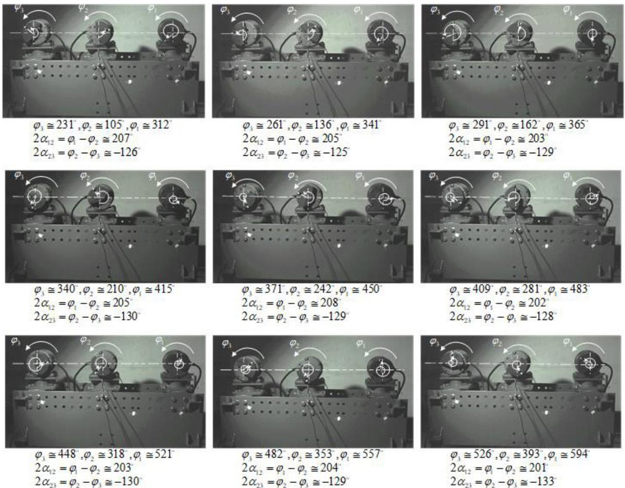
Fig. 10. Phase difference with three co-rotating rotors system
