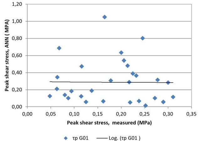
Fig. 7. Measured peak shear stress vs G01 model.
