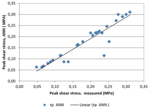
Fig. 6. Measured peak shear stress vs ANN predicted.
