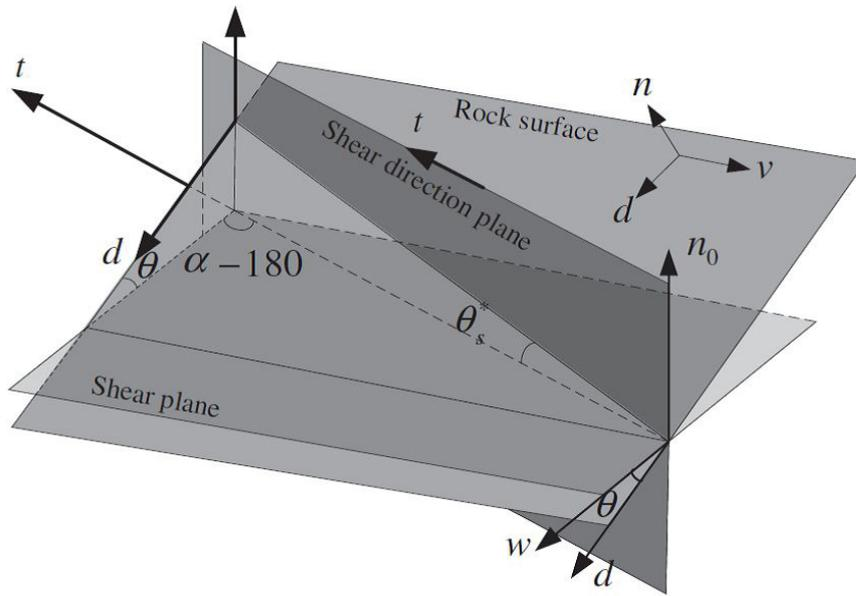
Fig. 5. Geometrical identification of apparent dip angle -  $\theta^*$ .
