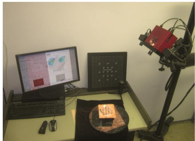
Fig. 3. The ATOS I 3D scanner and the sample.
