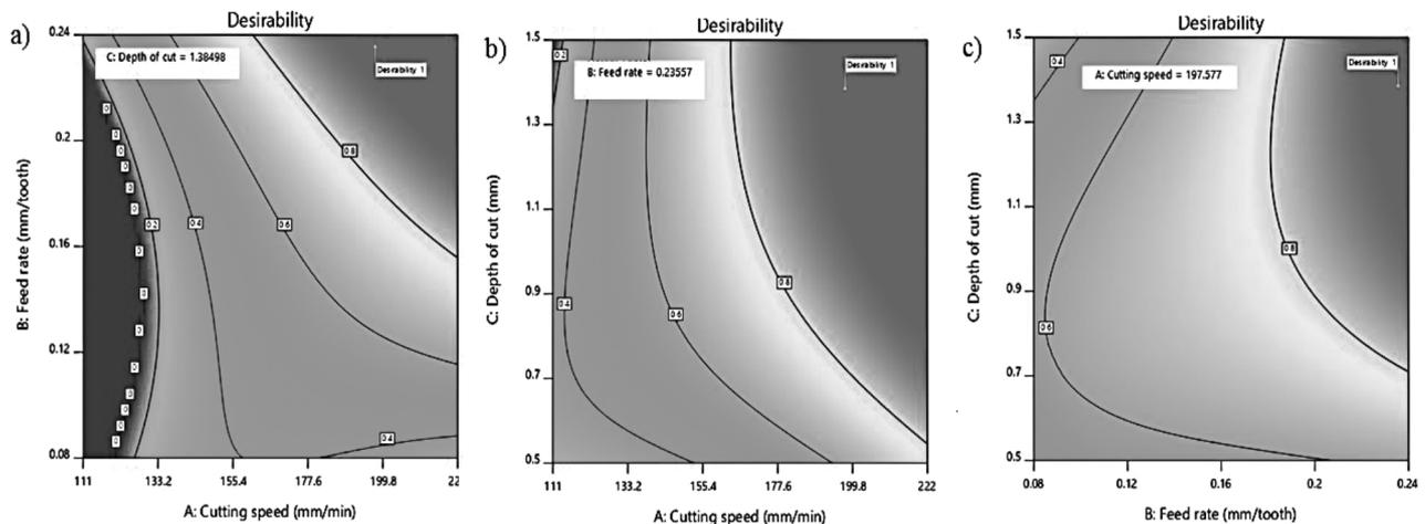
Figures 9: Contour plots for the overall desirability
