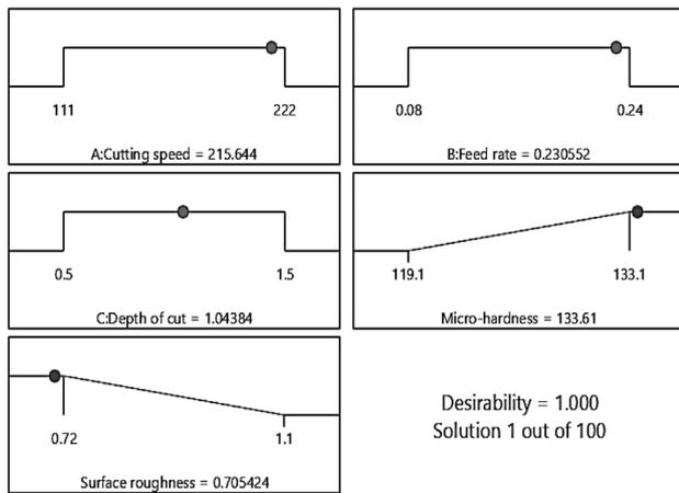
Figure 7: Ramp functions of process parameters and responses
