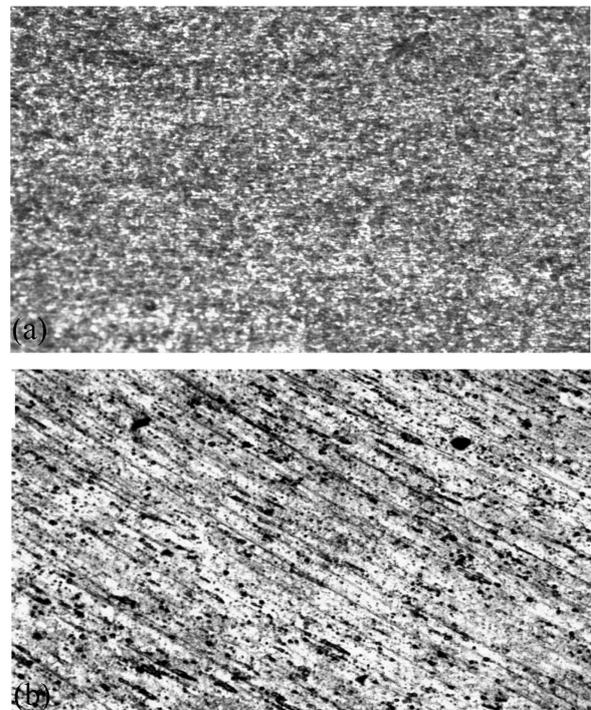
Figures 5: Microstructure of engine head: a) base metal, b) machined sample
