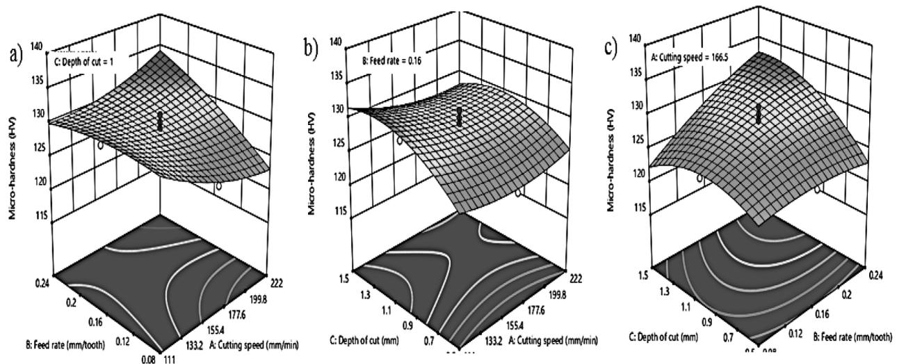
Figure 4: Interaction effects of the process parameters on the microhardness
