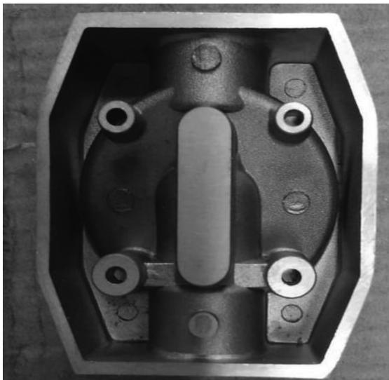
**Figure 2:** Face-milled diesel engine head
