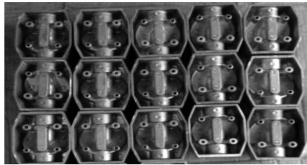
Figure 1: Pressure-die-casted diesel engine head
