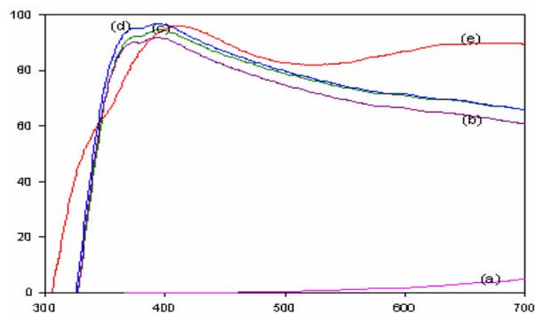
**Figure 7.** Optical transmission vs. wavelength of light for low tin doped  $\text{In}_2\text{O}_3$  thin film: (a) as-deposited, (b) annealed at 250, (c) 350 (d) 450, and (e) 550 °C.
