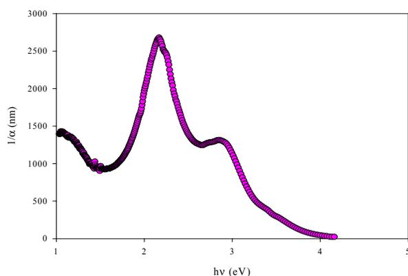
**Figure 8.** The adsorption depth variation vs incident photon energy.
