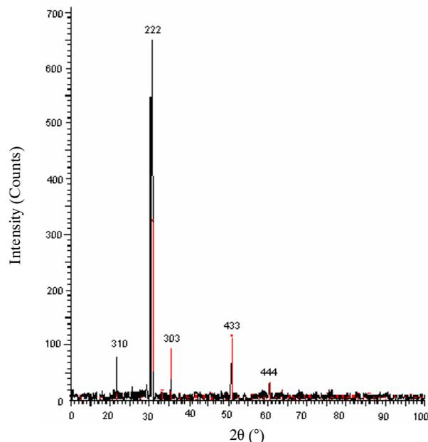
**Figure 6.** High angle-XRD pattern of tin doped  $\text{In}_2\text{O}_3$  sample after annealing at 550 °C. The bar graphs represents XRD pattern of  $\text{In}_2\text{O}_3$  sample.
