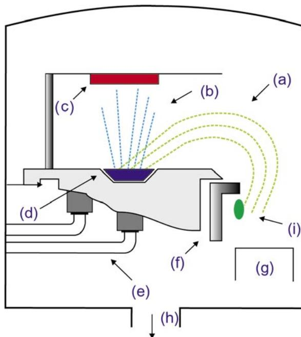
**Figure 1.** Electron beam evaporation set up used for thin films preparation; (a) Electron Beam, (b) Material Vapor, (c) Substrate, (d) Target Material, (e) Water Cooling Lines, (f) Shield, (g) Magnet, (h) To Vacuum Pump, (i) Tungsten Filament.
