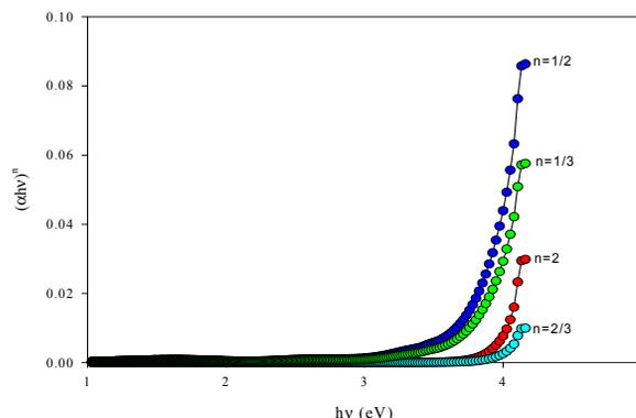
**Figure 9.** Comparison between allowed and forbidden direct and indirect transitions  $(\text{eV}\cdot\text{cm}^{-1} \times 10^4)^n$  in low level tin doped  $\text{In}_2\text{O}_3$  thin film heated at 550 °C for 24 h.
