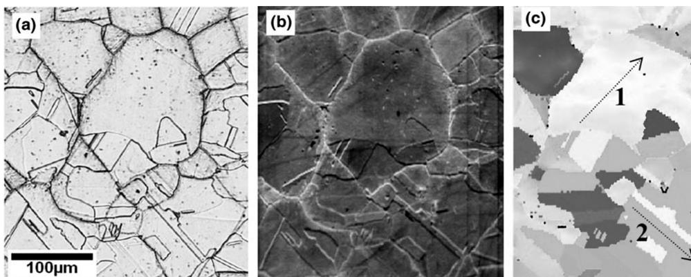
**Figure 2:** Analysis of the microstructure with: a) optical microscopy, b) secondary electron microscopy image, c) EBSD<sup>3</sup>
