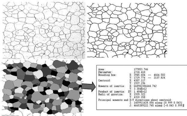
Figure 4: Schematic representation of the steps of digital imaging and the calculated result for one grain
