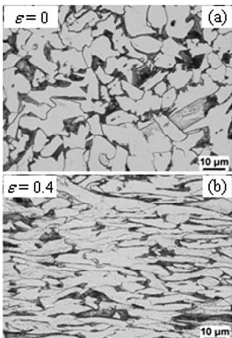
**Figure 1:** Microstructures of the C-Mn steel: a) the initial state; b) the microstructure after a deformation<sup>1</sup>
