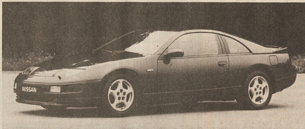
Nissan 300 ZX, trilitrski motor V6, 24 ventilov, 280 KM, 250 km na uro
