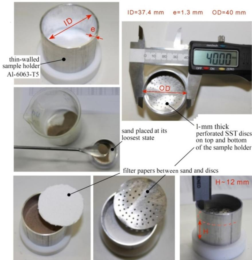
Figure 3. Sample preparation of the one-dimensional compression tests.
