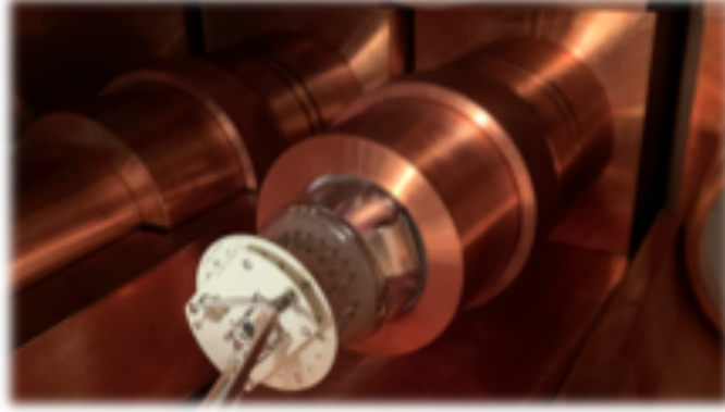
Fig. 2.4: Picture of the voltage divider plus preamplifier system connected to the flying leads of a PMT in DAMA/LIBRA-phase2-empowered during installation in HP Nitrogen atmosphere.
