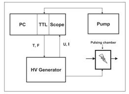
**Figure 1.** Configuration of a flow through electropulsator. The TTL trigger drives the delivery of the pulse with a preset duration and frequency. The voltage is set on the generator. All signals are monitored on line on the oscilloscope and the PC. The flow rate is adjusted with a peristaltic pump.
