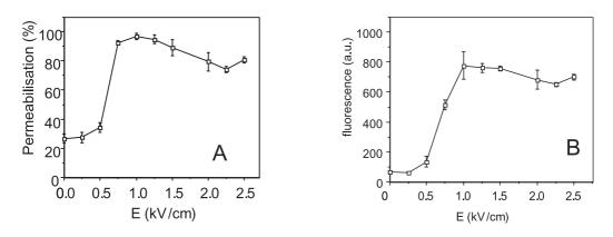
**Figure 2.** Control by the field on cell permeabilization. CHO cells ( $10^6$  per ml) were treated by a train of 10 pulses lasting 1 ms at a frequency of 1 Hz with a flow rate of 1.2 ml/min. The pulsing buffer contains the hydrophilic dye PI. Permeabilization is assayed by the number of fluorescent cells (A) and by the mean fluorescence emission of the population (B) by use of a flow fluocytometer.
