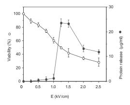
**Figure 6.** Electrorelease of cytoplasmic proteins. CHO cells ( $10^6$  per ml) were treated by a train of 10 pulses of 1 kV/cm lasting 1 ms at a frequency of 1 Hz with a flow rate of 1.2 ml/min. Their viability was assayed 24 h after the treatment by the crystal violet test. The data were corrected from the effect of the flow on the control cells, which brought a 30% loss.
