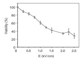
**Figure 3.** Viability of pulsed cells. CHO cells ( $10^6$  per ml) were treated by a train of 10 pulses lasting 1 ms at a frequency of 1 Hz with a flow rate of 1.2 ml/min. Their viability was assayed 24 h after the treatment by the crystal violet test. The data were corrected from the effect of the flow on the control cells, which brought a 30% loss.
