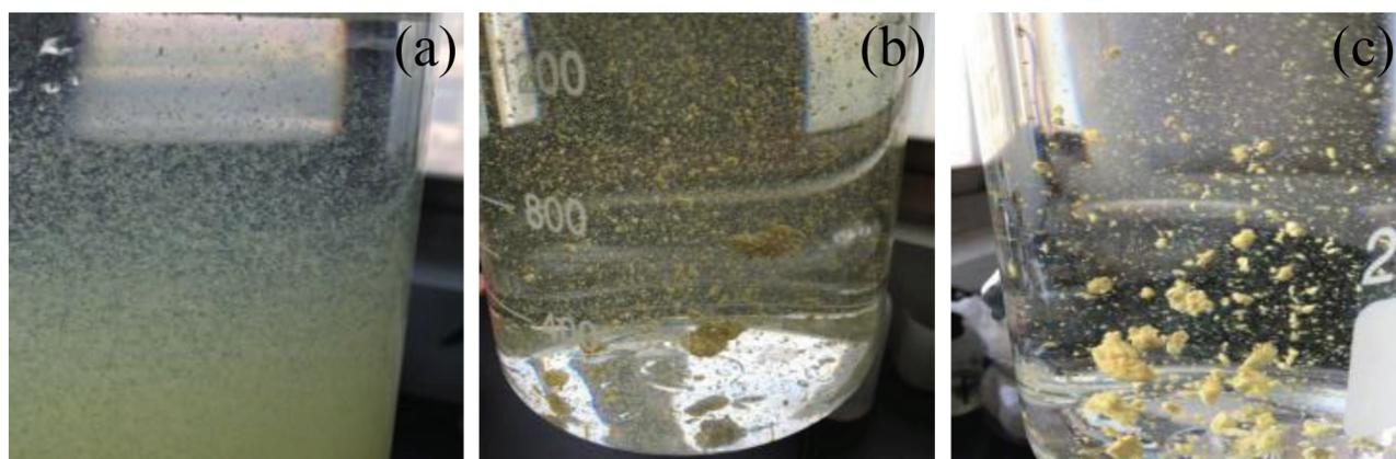
**Figure 3:** Observation of flocculation morphology: a) ATP, b) CS, c) ATP/CS
