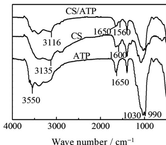
Figure 1: FTIR spectra of ATP, CS and CS/ATP
