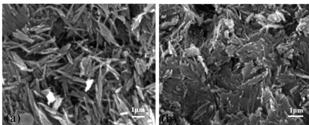
Figure 2: SEM micrographs of: a) ATP, b) CS/ATP
