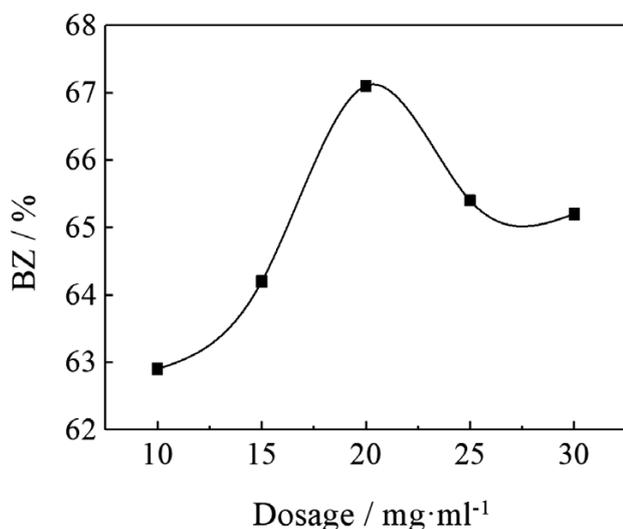
**Figure 6:** Effect of the flocculant dosage on the BZ content in the waste solution
