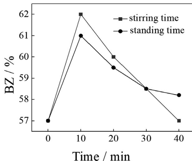
**Figure 7:** Effect of the stirring and standing time on the BZ content in the waste solution
