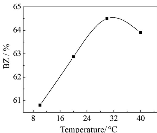
**Figure 5:** Effect of the flocculation temperature on the BZ content in the waste solution
