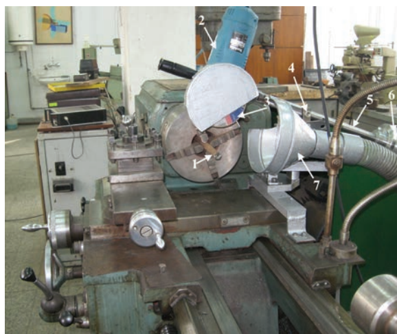
Fig. 2. Work stand for elastic abrasive cutting
