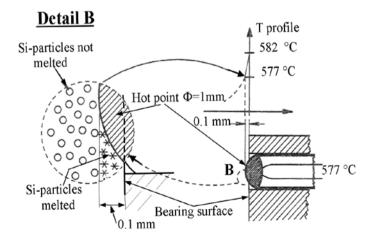
**Figure 2.** The basic principle of the previously way of temperature measurement on the bearing surface of die in aluminium hot extrusion<sup>[5]</sup>.
