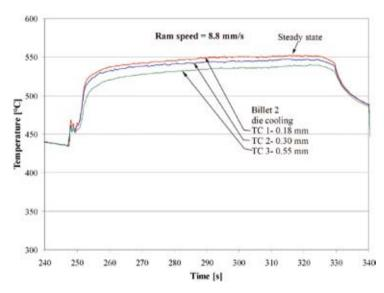
**Figure 7.** Time course of measured values of temperature in the die for different distances from the bearing surface, billet No. 2, ram speed=8.8 mm/s, die cooling (N<sub>2</sub>).
