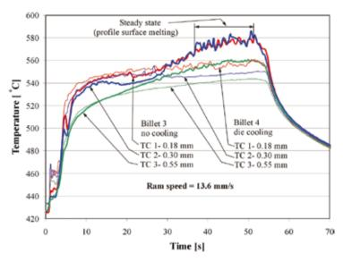
**Figure 8.** Comparison between the measured temperatures on the die bearing surface during extruding of the billet No. 3 and of the billet No. 4.
