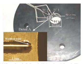
Figure 4. Dividing surface of split die used with channels made for embedding and welding
