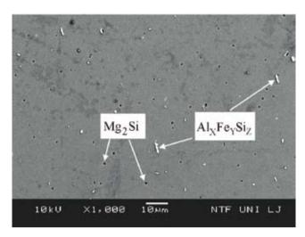
**Figure 5.** BEC image of homogenized initial billet microstructure; distribution of Mg<sub>2</sub>Si and AlFeSi particles across the cross-section of the billet visible.
