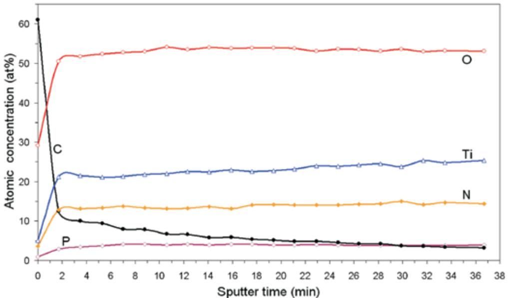
**Figure 3.** AES depth profile of unused titanium medical implant with golden colour protective layer
