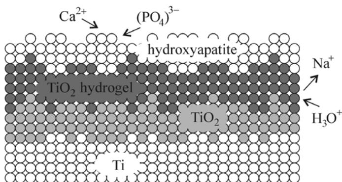
**Figure 5.** A formation of calcium phosphate rich layer on titanium oxide film
