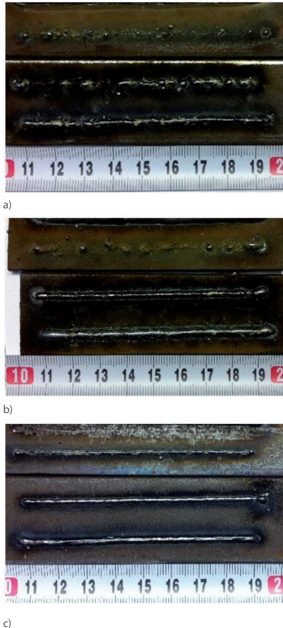
Figure 2: Welding at 40 A a) standard, b) pulse and c) CMT (different welding speeds from bottom to top: 3, 7.5 and 12 mm/s).
