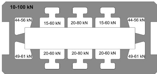
Fig. 8. Ranges for the holding forces
