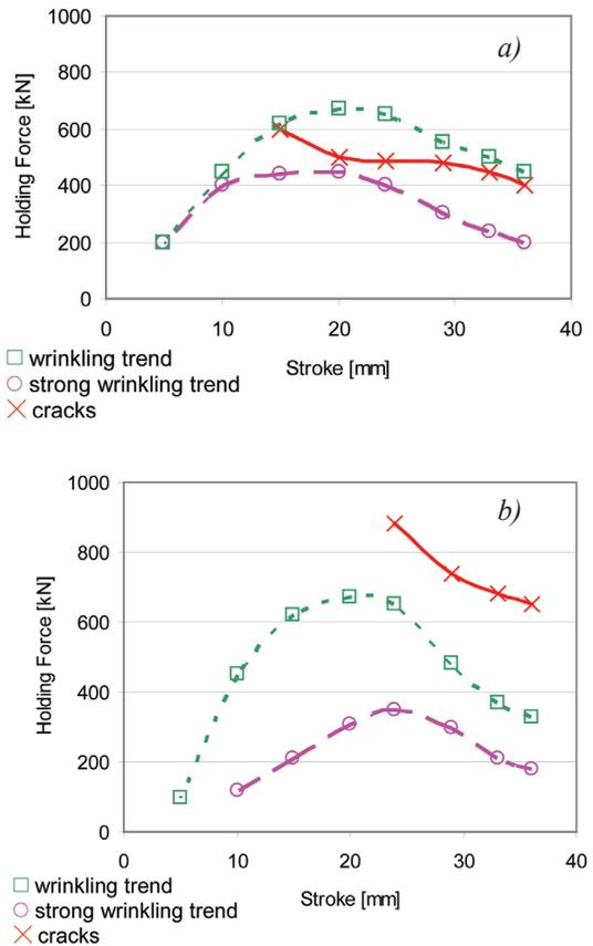
Fig. 9. Technological window for a) conventional holding system and b) segmented holding system
