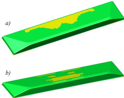
Fig. 7. Good workpieces made by segmented holding system a) with segmented holding forces 306 kN b) with segmented holding forces 734 kN
