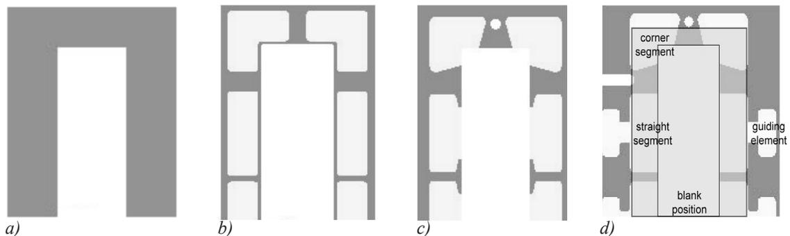
Fig. 5. a) Conventional blankholder and b), c), d) three versions of segmented blankholder
