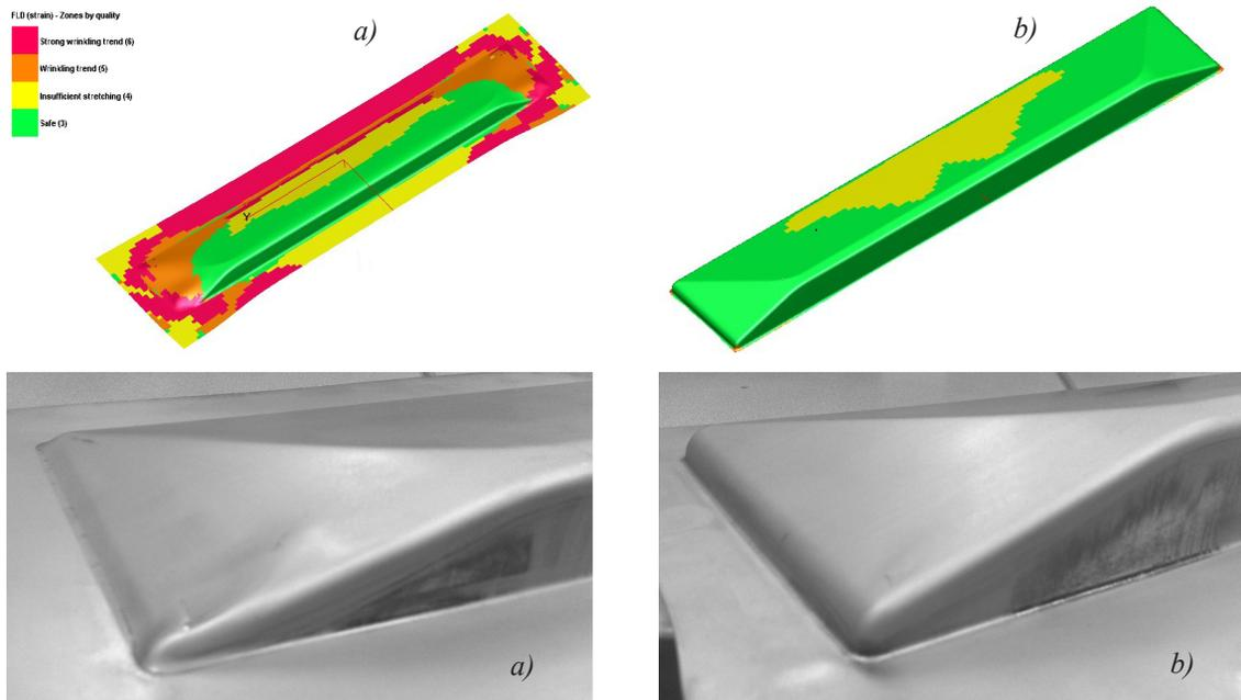
Fig. 11. Wrinkling trend; a) step 4 (FEM), b) step 10 (FEM), c) early step (experiment) and d) final draw (experiment)
