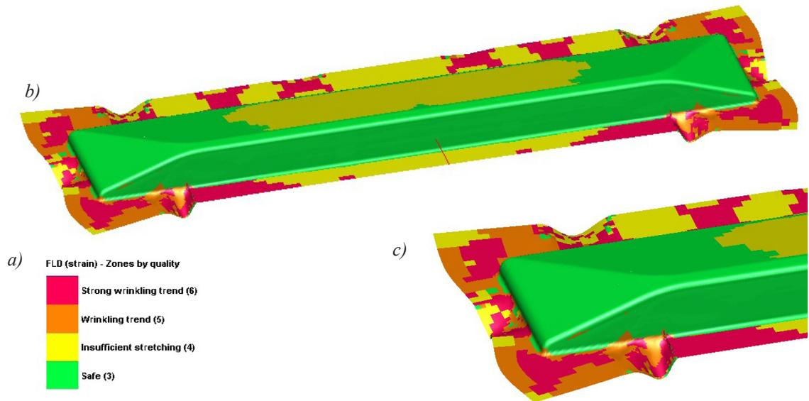
Fig. 6. Flange wrinkling; a) whole model, b) colour scheme, c) detailed view
