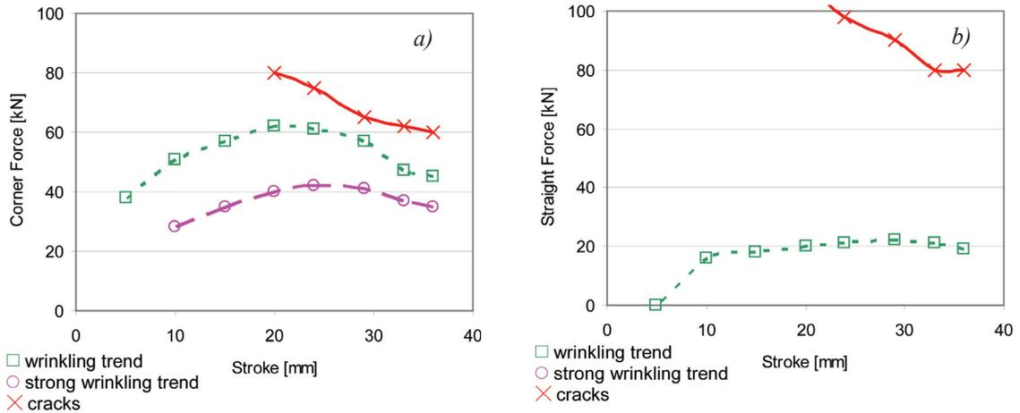
Fig. 10. Technological window for; a) corner areas and b) straight areas
