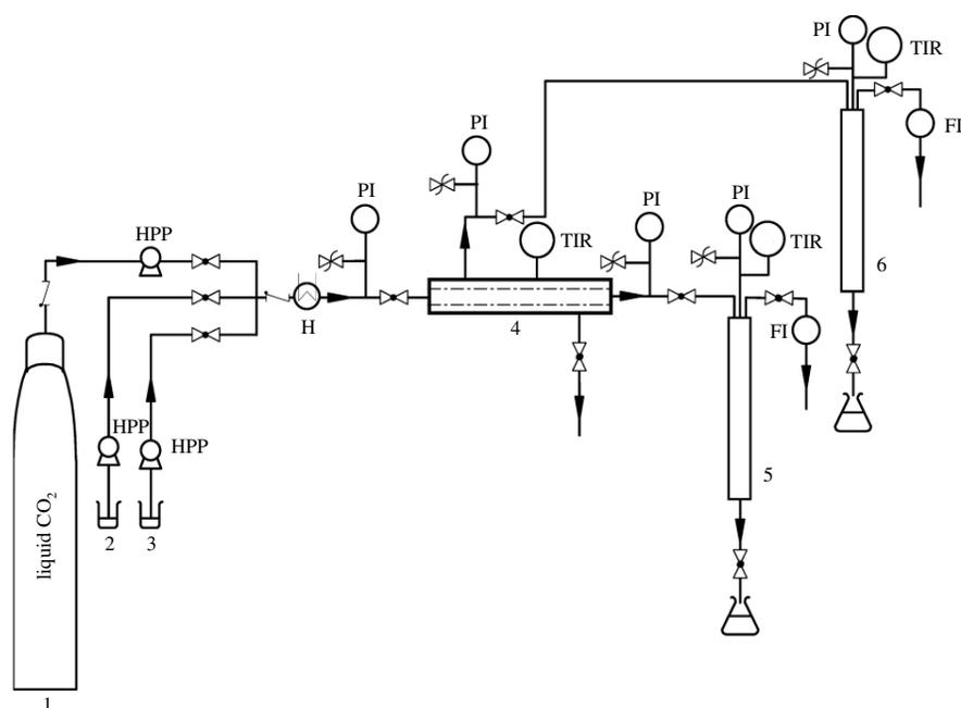
**Figure 7:** High-pressure continuous enzymatic tubular membrane reactor; 1 – gas, 2, 3 – substrates, 4 – membrane reactor with ceramic tubular membrane, 5, 6 – separation columns, HPP – high pressure pump; TIR – temperature regulator and indicator; P – pressure indicator; FI – flow indicator.
