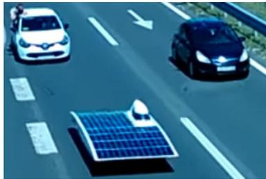
Figure 5: Testing of the CROsolar01 solar electric car in realistic road condition.
