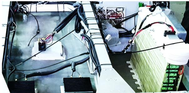
Figure 3: EMC problem of an inductive and capacitive coupling in electric circuits of solar electric car prototype CROsolar01.
