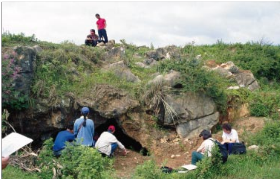
Photo 1: On September 26, 1997 we injected 1 kg of uranine at Point 6 - Wayadong. Foto 1: Dne 26. septembra 1997 smo injicirali 1 kg uranina na točki 6 - Wayadong.
