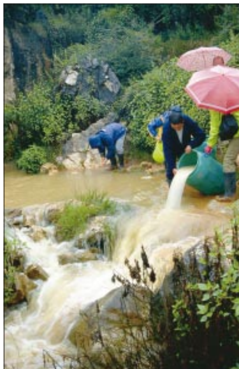
Photo 1: On September 26, 1997 we injected 1 kg of uranine at Point 6 - Wayadong. Foto 1: Dne 26. septembra 1997 smo injicirali 1 kg uranina na točki 6 - Wayadong.
