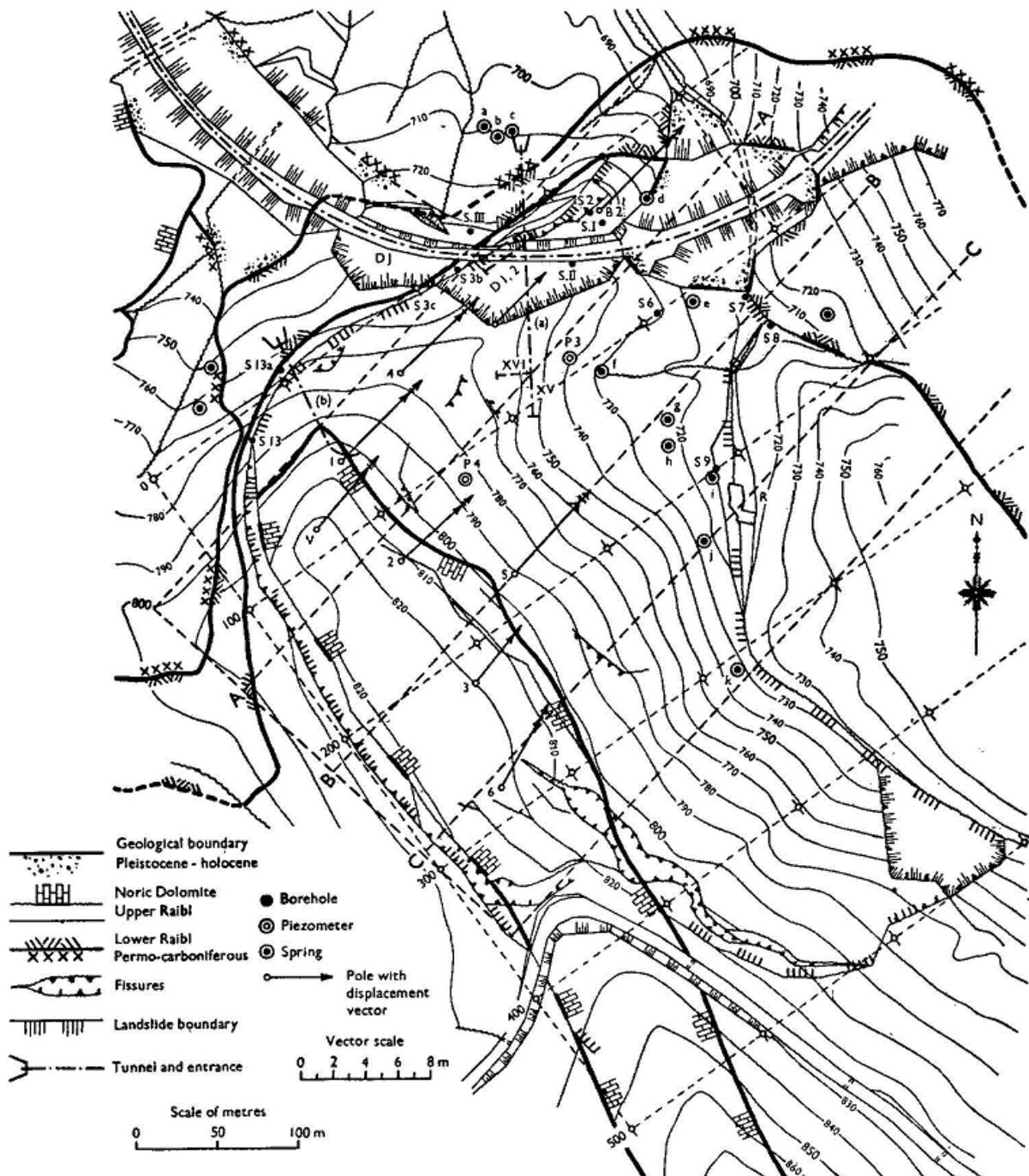
Figure 4. Mapping the Zalesina Landslide, Croatia, (Republika Hrvatska) [8].
