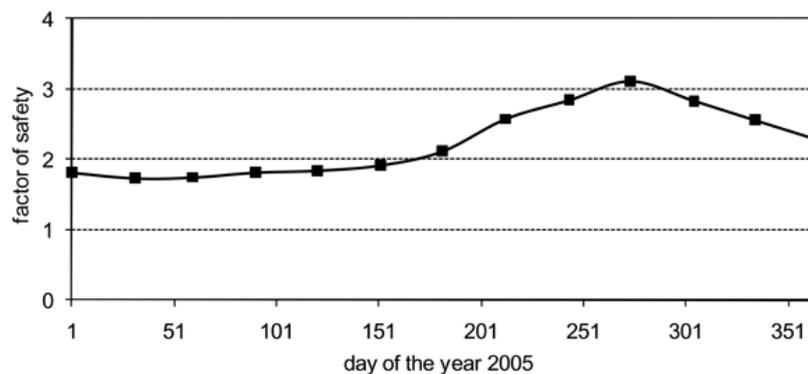
**Figure 22.** Tössegg: seasonal variation of factor of safety in 2005 against slope failure calculated using SLOPE/W after coupling with suctions and pore pressures obtained from TH Modelling with VADOSE/W (after [58]).
