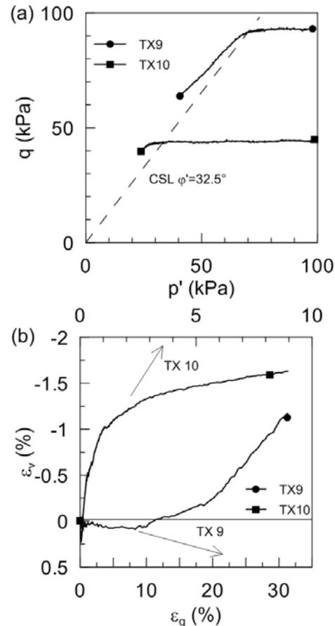
**Figure 17.** Anisotropic consolidation drained shear under constant axial load (CADCAL) triaxial stress path tests on reconstituted Rüdlingen silty sand: (a) stress path data shown in  $q$ - $p'$  space; (b)  $\epsilon_q$ - $\epsilon_v$  space, with strain axes at the top of TX10 and bottom for TX9 [80].
