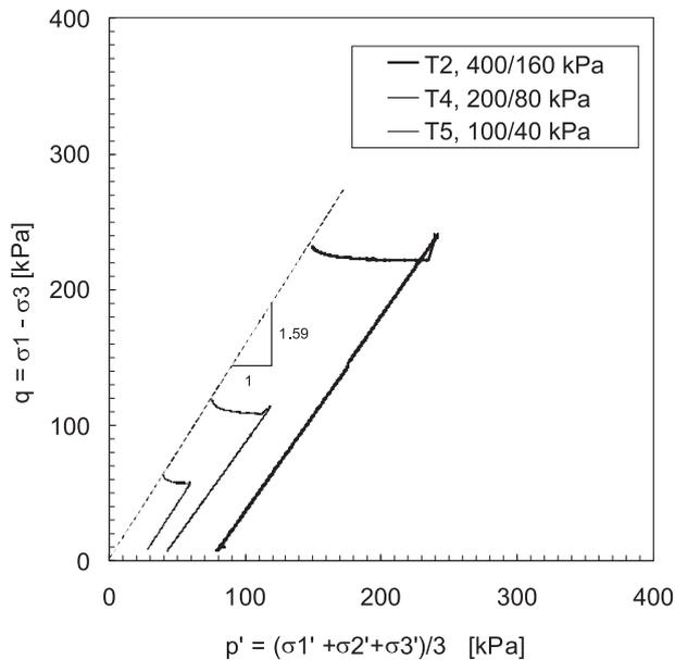
**Figure 16.** Constant Shear Drained (CSD) triaxial stress path tests on reconstituted Gruben moraine: stress path data shown in  $q$ - $p'$  space with consolidation to  $\sigma_1'/\sigma_3'$  as shown in the legend, prior to shear (after [71]).
