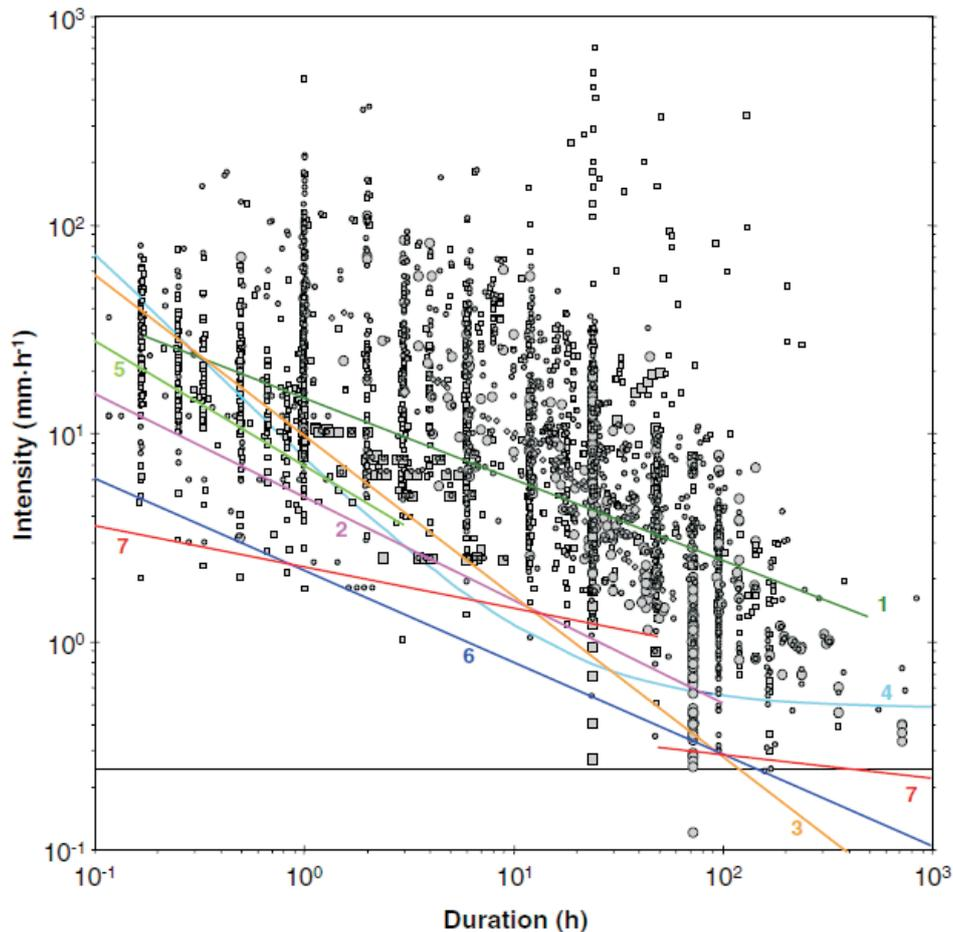
**Figure 5.** Global Intensity-Duration thresholds based on Guzzetti et al., [26] with published global (worldwide) Intensity-Duration rainfall thresholds proposed by: 1 [25]; 2 [27]; 3 [28]; 4 [29]; 5 [30]; 6 Inferred from this data; 7 thresholds inferred from the probability estimates of the rainfall conditions, for two different rainfall periods ( $D < 48$  h,  $D \geq 48$  h). The horizontal line shows a 0.25-mm/h rainfall intensity.
