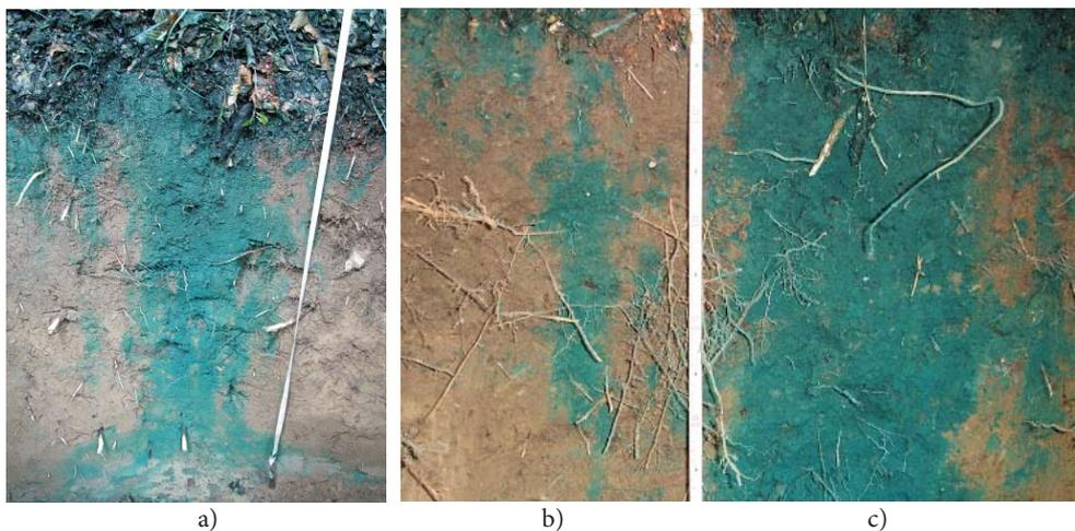
**Figure 12.** Rüdlingen: excavation of pits following infiltration tests (a) primarily vertical flow with lateral spreading above rock [79], (b) indications of partially saturated flow (c) root matrix (photographs: Dr. Peter Kienzler).
