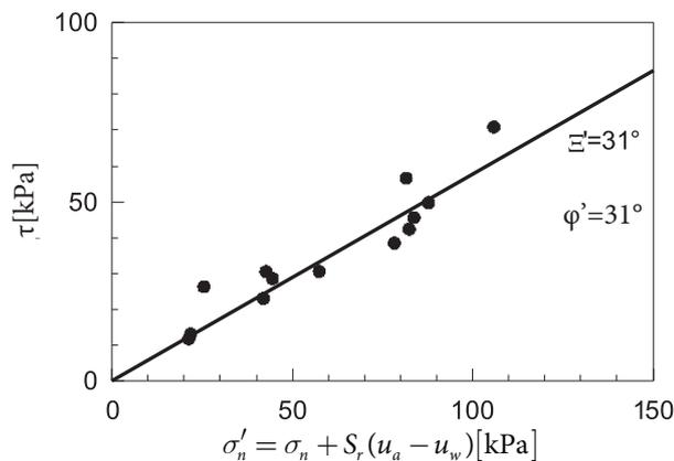
**Figure 21.** Rüdlingen: Interpretation of direct shear tests at constant water content to predict the critical state angle of friction for the reconstituted silty sand [100].
