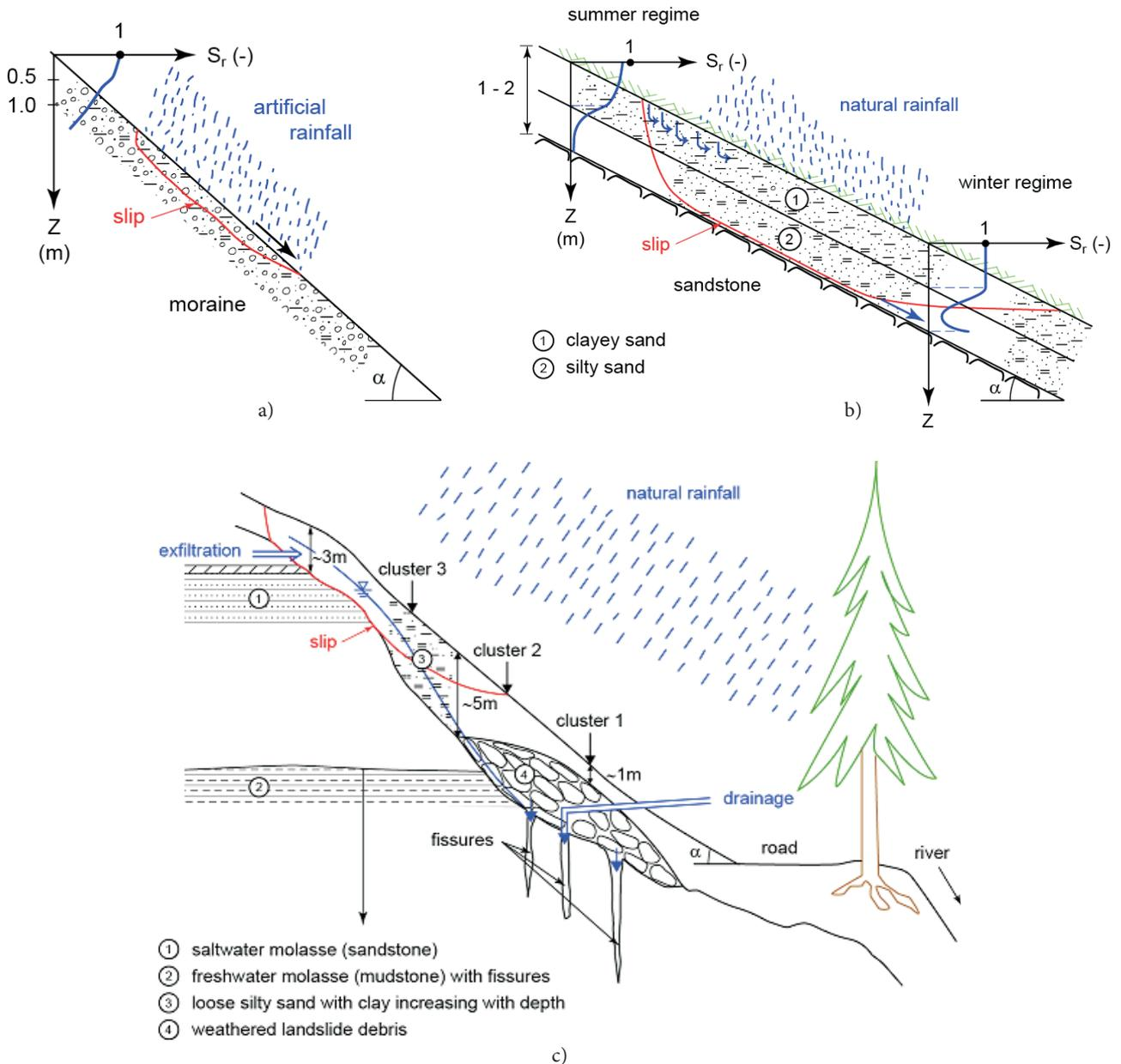
**Figure 15.** Saturation mechanisms after Springman [86] with a) ,top down' saturation through infiltration, typically moraine as in Gruben [57,71]; b) in summer regime ,top down', in winter regime additional ,bottom up' through run-off above bedrock, as for Tössegg [76]; c) exfiltration from and infiltration into underlying rock at Rüdlingen (sketch interpreted from [60]).
