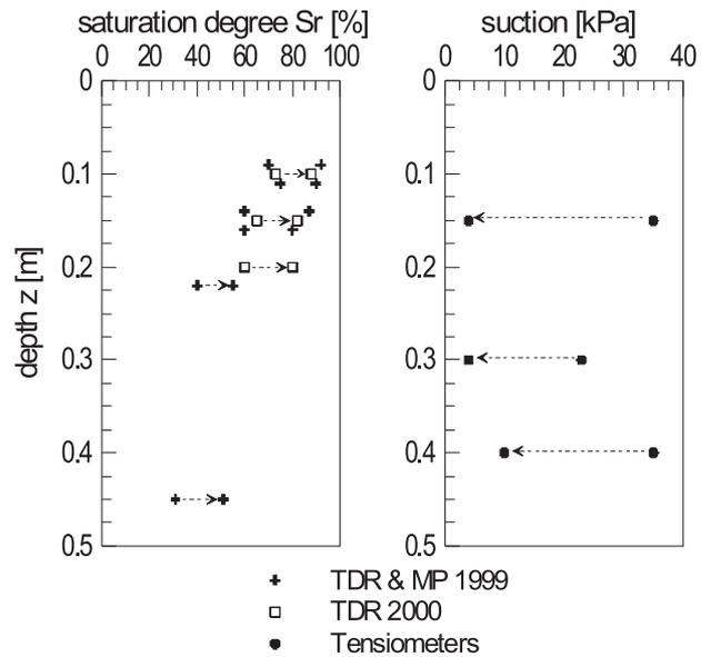
**Figure 8.** Gruben: summary of immediate pre- and post-rainfall event data showing increase in saturation combined with loss of suction as infiltration progresses (a) saturation degree determined from TDR and MP probes: Fields 1/1999 & 1/2000 (31° slope), (b) Suctions determined from tensiometers: Field 1/2000 (31° slope), Gruben [71].
