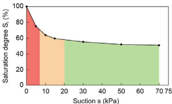
**Figure 24.** Relationship between saturation degree and suction of Rüdlingen silty sand in the laboratory based on the wetting branch of the Water Retention Curve [80] superimposed with alarm levels [86].
