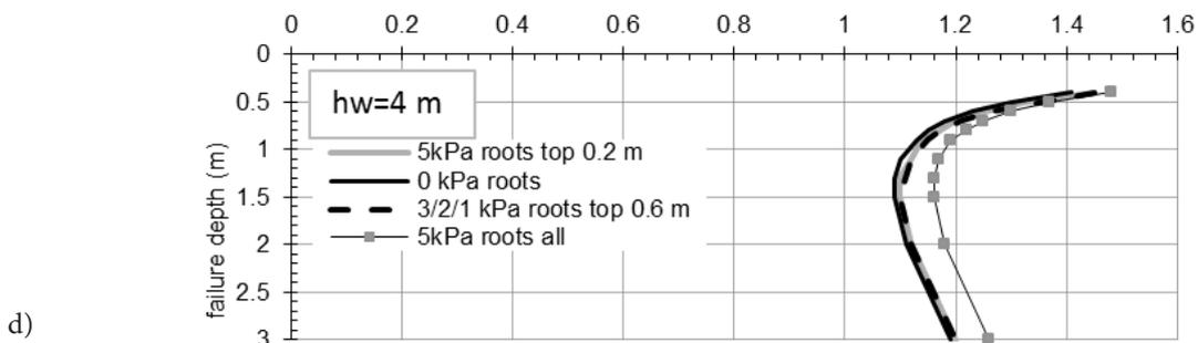
**Figure 23.** Two-dimensional limit equilibrium stability calculations for a channel geometry, including suctions (when above the water table) and root reinforcement on the sides and base: (a) channel dimensions with parameters appropriate for Rüdlingen; results for various values of  $c_r$  and water tables at (b)  $z = 0.8\text{ m}$  (c)  $z = 1.2\text{ m}$  (d)  $z = 4\text{ m}$ .
