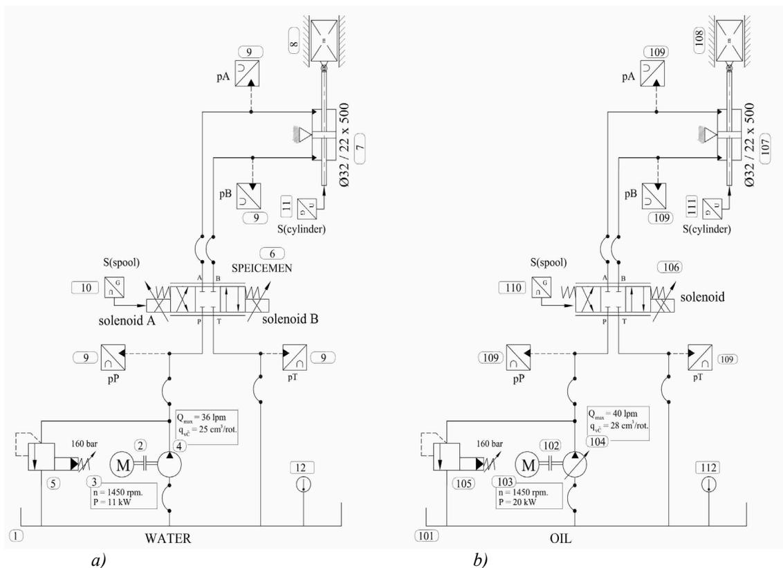
Fig. 1. Hydraulic circuits of the test rig
