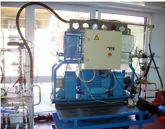
Fig. 3. Oil power-control part of the test rig
