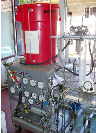
Fig. 2. Water power-control part of the test rig
