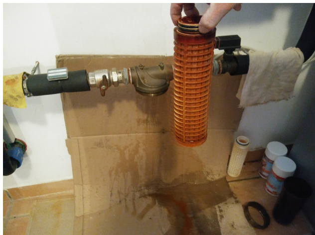
Fig. 4. Iron mineral deposits on heat pump filter from northern part of Ljubljansko barje.
