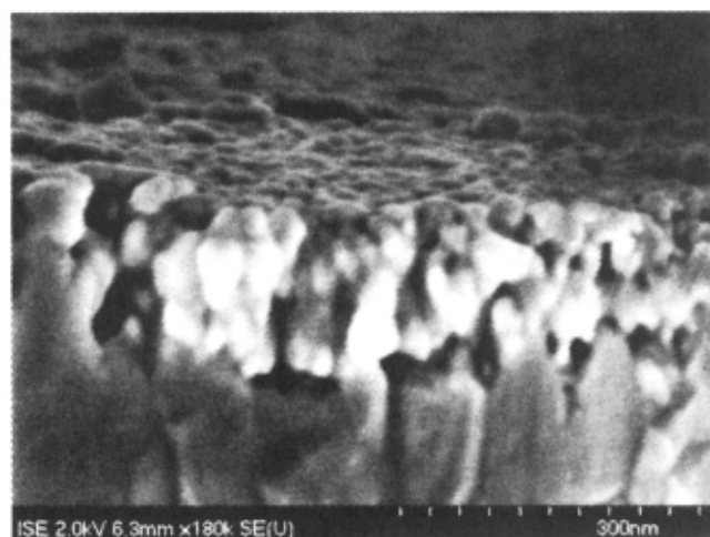
Slika 8: SEM-posnetek plasti \text{CoCuMnO}_x -II
