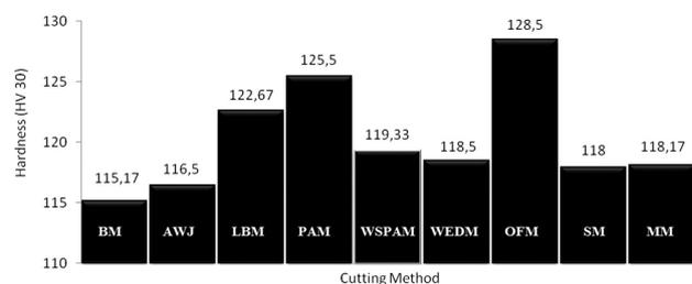
**Figure 11:** Comparison of the hardness values for the brass-353 ( $\alpha+\beta$ ) samples cut with different methods in comparison with the original hardness of the material core
