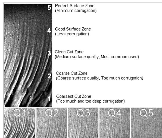
Figure 3: Cut-face quality zones based on jet flow<sup>1,43</sup>
