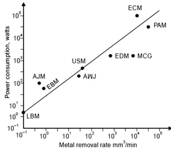
**Figure 6:** Comparison of the abrasive water jet with the other cutting methods<sup>2,9,13</sup>
