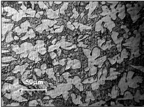
**Figure 8:** Microstructure of brass-353 ( $\alpha+\beta$ )
