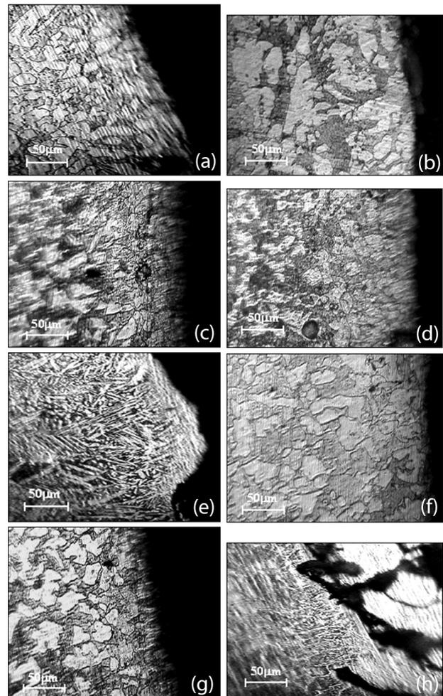
**Figure 9:** a) Stripe-saw cutting, b) milling cutting, c) underwater plasma cutting, d) laser cutting, e) plasma cutting, f) abrasive water jet cutting, g) wire-erosion cutting, h) oxygen-flame cutting
