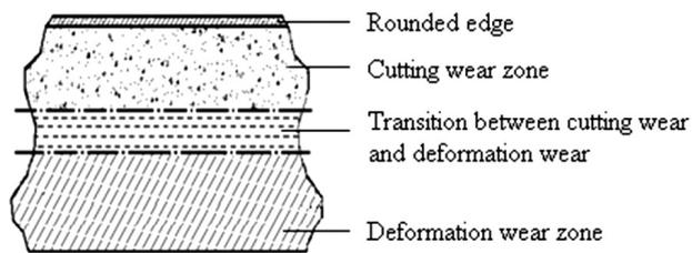
Figure 2: Surface sections cut by the abrasive water jet<sup>4</sup>
