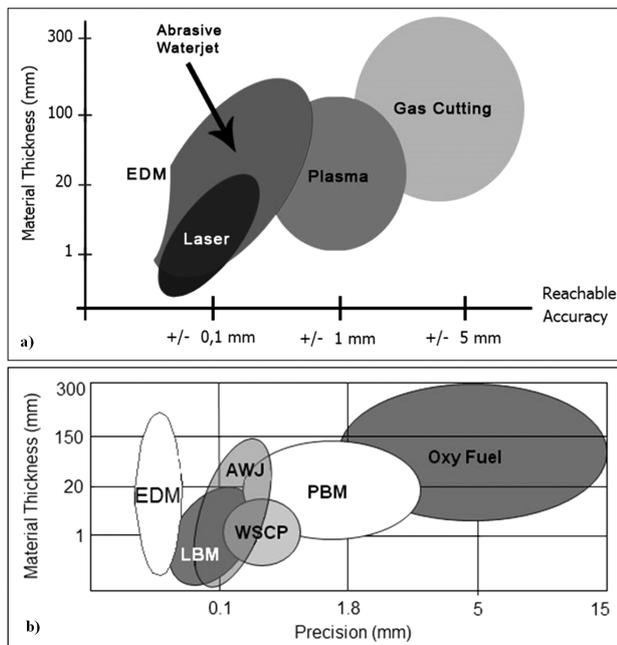
**Figure 5:** Comparison of the abrasive water jet with the other cutting methods<sup>4,8</sup>
