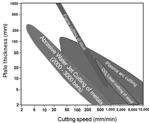
**Figure 4:** Comparison of the cutting abilities of different cutting methods using single-orifice jet beams<sup>8</sup>
