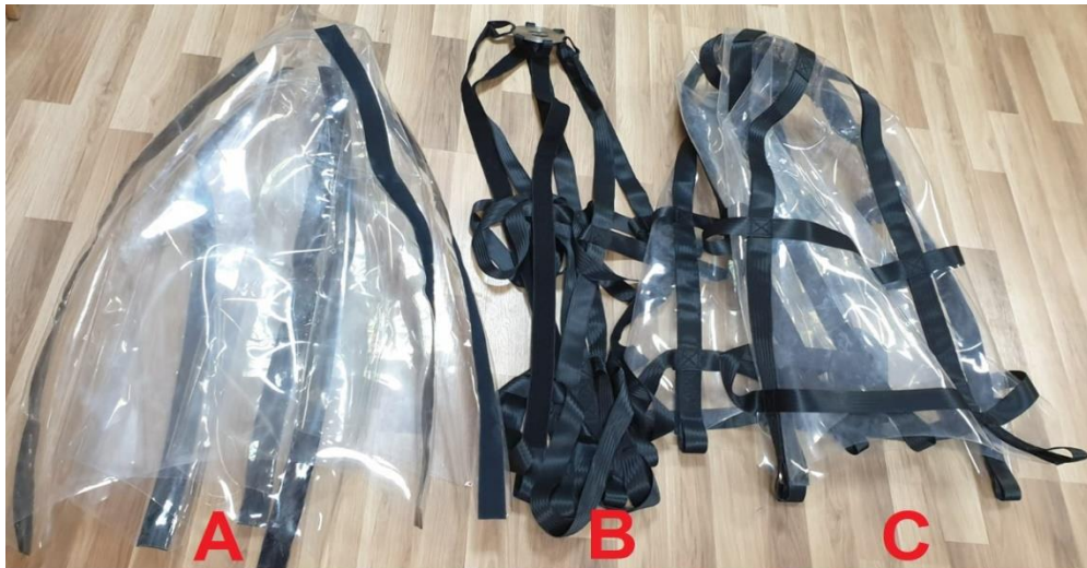
Figure 2: Batychron main components A) transparent dome, B) openwork mesh, and C) flexible diving bell – the Batychron. P.Kolakowski. 2022.
