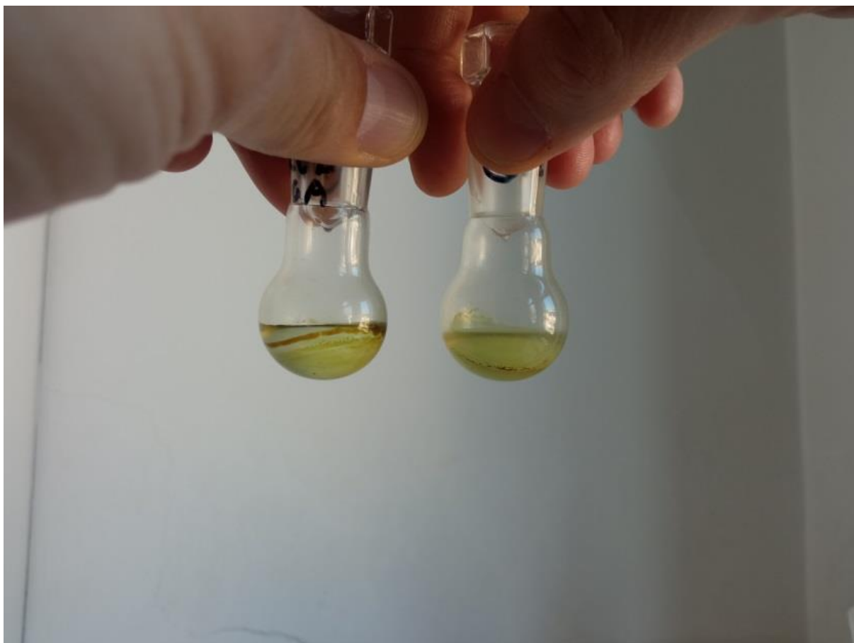
Figure 2: Comparison in water solubility between unmodified (left) and modified (right) hemp resin. Mitja Križman and Jure Zekić. 2022.
