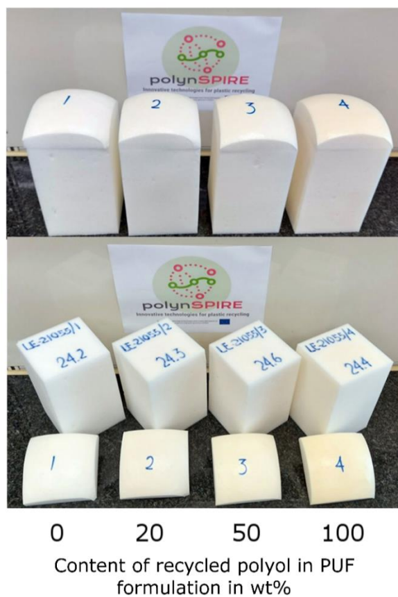
Figure 2: The high quality of recycled polyols produced by our method was confirmed by Repsol in Spain, a multinational company that produces commercial polyols for the synthesis of polyurethanes. Repsol synthesized flexible PUFs that were tested for their mechanical properties. The mechanical properties of PUFs made from our recycled polyols are comparable to PUFs made from virgin polyols. Company Repsol. 2021.
