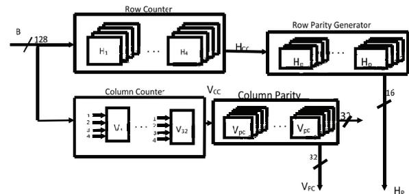
Figure 2: Architecture for CMC Encoder.
