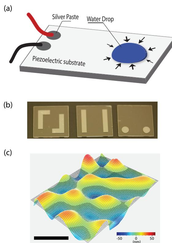
**Figure 1:** (a) Schematic illustration and (b) images of various electrode patterns on the lithography-free  $\text{LiNbO}_3$  chip. (c) Laser Doppler Vibrometer (LDV) scan of the chip at 3.5 MHz; the scale bar denotes a length of approximately 1 mm.
