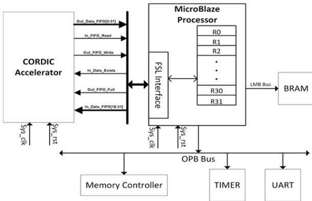
**Figure 5:** CORDIC Accelerator with MicroBlaze Processor System
