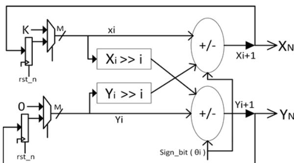
**Figure 6:** Standard CORDIC Hardware Accelerator Block
