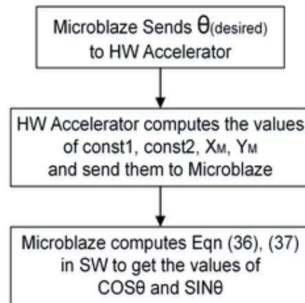
**Figure 10:** Flow chart for Modified CORDIC Accelerator Implementation
