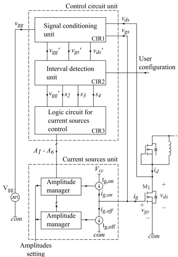
Figure 3: Advanced gate control system block diagram
