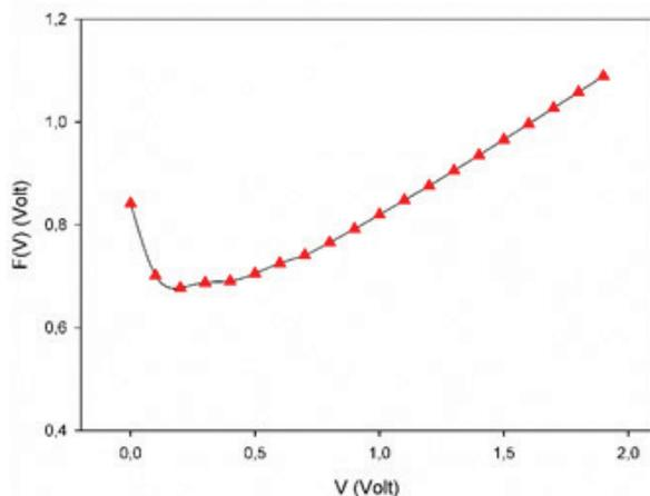
**Figure 4:** Plot of Norde function;  $F(V)$  vs.  $V$
