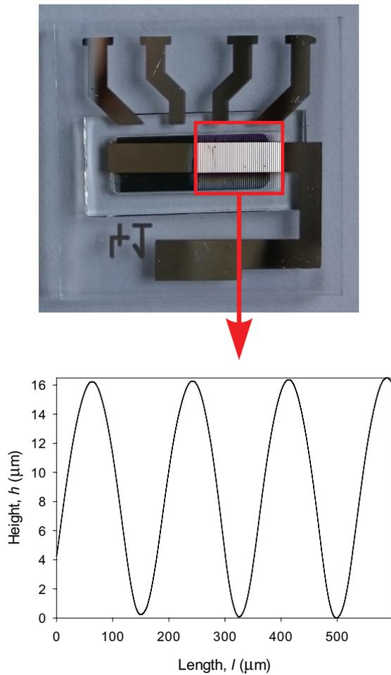
**Figure 5:** A produced bottom-emitting red OLED (four dots as indicated by the contacts) with sine textures on glass / air interface. Red rectangle indicates limited textured area of approx. 7x9 mm<sup>2</sup>. Additionally, profilometer measurements of the sine textures for selected example is also shown.
