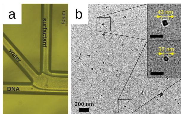
**Figure 5:** Assembly of DNA-based nanoparticles by slow diffusion. (a) Optical image of the microfluidic device. (b) Transmission electron microscopy images of DTAB-DNA nanoparticles. The scale bars of insets are 100 nm. Adapted with permission from [33]. Copyright 2015 American Chemical Society.
