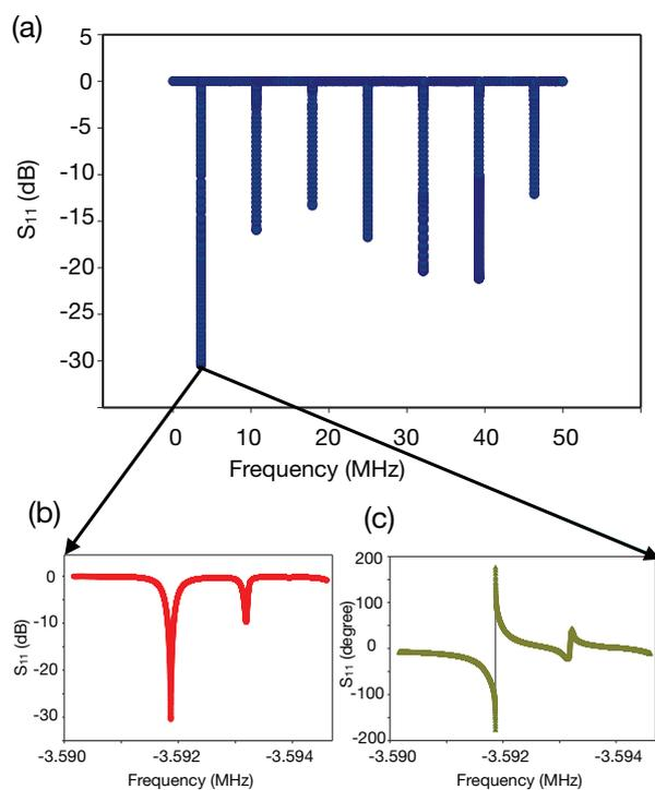
**Figure 2:** (a) Results from the VNA frequency sweep to measure the insertion loss parameter  $S_{11}$  of the device, which clearly shows multiple resonances starting from the fundamental resonance at 3.5 MHz, as determined from the magnification of (b) the magnitude and (c) the phase angle, and higher harmonics at every additional 7 MHz.
