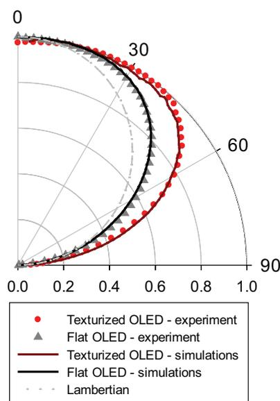
**Figure 7:** Angular intensity distribution (AID) comparison for flat and device with textured interface (sine textures on interface substrate/air with  $P = 175 \mu\text{m}$  and  $h = 15 \mu\text{m}$ ) vs. simulation results for corresponding structures. Additionally, ideal Lambertian distribution is added.
