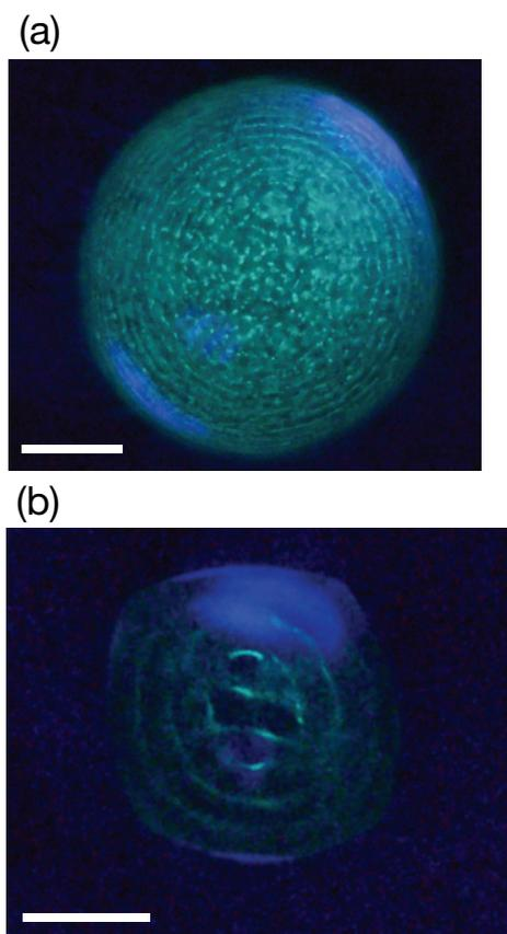
**Figure 4:** Top view of the three-dimensional concentric particle patterns that arise under Lamb wave substrate excitation of (a) a circular, and, (b) a roughly square 5  $\mu\text{l}$  sessile liquid drop comprising 3  $\mu\text{m}$  particles suspended in water at 10.5 MHz. The spacing between the concentric rings is approximately 90  $\mu\text{m}$ . Scale bars denote a length of typically 1 mm.
