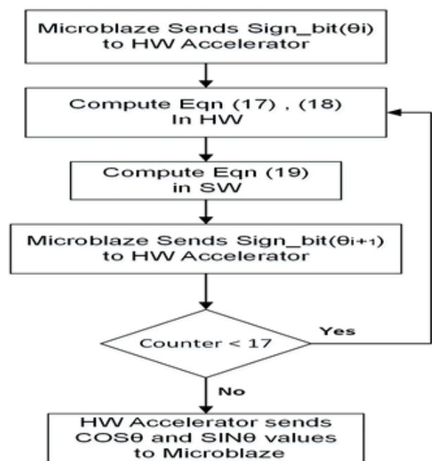
**Figure 7:** Flow chart for Standard CORDIC Accelerator Implementation
