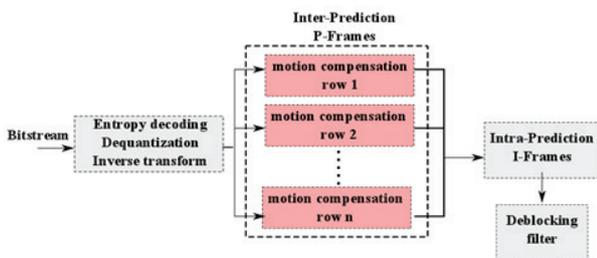
**Figure 3:** Parallel motion compensation application block diagram
