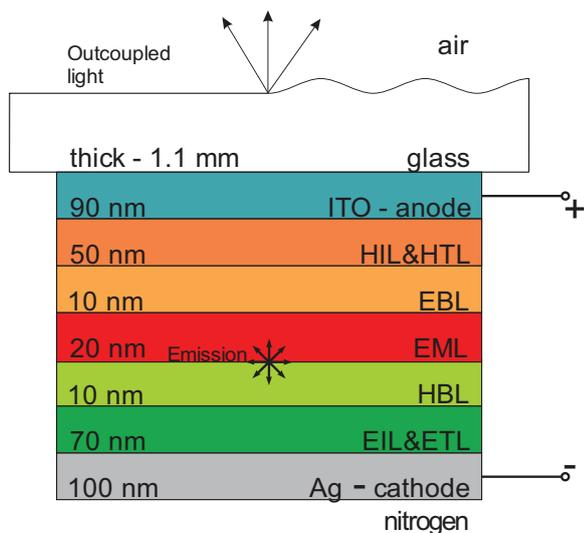
**Figure 1:** Structure of a conventional p-i-n bottom-emitting red OLED deposited on a glass substrate and encapsulated under a nitrogen atmosphere. Texturization of the substrate (on light escaping side) is indicated on the right hand side of the substrate.
