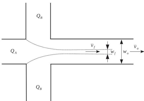
**Figure 3:** Schematic illustration of hydrodynamic flow focusing in a microfluidic device.  $Q_A$  and  $Q_B$  are the flow rates of the central and lateral streams respectively,  $w_f$  and  $w_o$  denote the width of the focused and outlet streams, and  $v_f$  and  $v_o$  are the average flow velocities in the focused and outlet streams. Adapted with permission from [31]. Copyright 2014 American Chemical Society.
