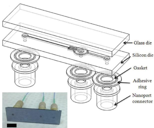
**Figure 4:** Microfluidic device for hydrodynamic flow focusing with an exploded view showing the various parts made in a combination of glass and silicon. The photograph shows the bottom of the device. The scale bar is 1 cm. Adapted with permission from [32]. Copyright 2013 American Chemical Society.
