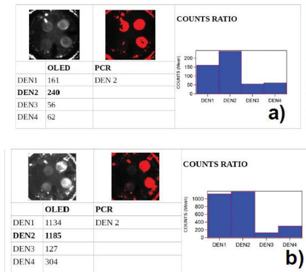
**Figure 2:** Fluorescence image acquired with the CCD camera and the same image with threshold applied, to outline the brightest spots: a) anti-NS1 IgM detection with NS1 spots deposited as shown in Fig. 1, b) anti-NS1 IgG detection with NS1 spots deposited as shown in Fig. 1.
