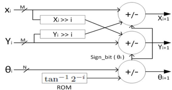
Figure 3: Internal implementation of Standard CORDIC PE
