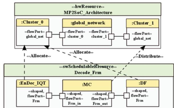
**Figure 7:** Allocation for the motion estimation parallelization
