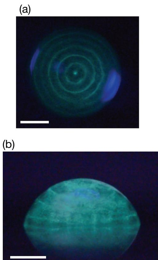
**Figure 3:** (a) Top and (b) side view of the three-dimensional concentric particle patterns that arise under Lamb wave substrate excitation of a 5  $\mu\text{l}$  sessile liquid drop comprising 3  $\mu\text{m}$  particles suspended in water at the fundamental resonant frequency, i.e., 3.5 MHz. The spacing between the concentric rings is approximately 270  $\mu\text{m}$ . Scale bars denote a length of approximately 1 mm.
