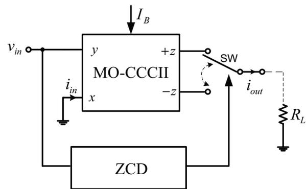
**Figure 1:** The proposed circuit of the full-wave rectifier
