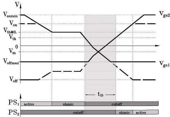
Figure 3. Basic mirrored control voltages marked with a dotted line and actual gate-source voltages including a -4 V clamping and a 5 V increase with a solid line. The stages of the power devices  $PS$  and the  $t_{ID}$  are marked below.
