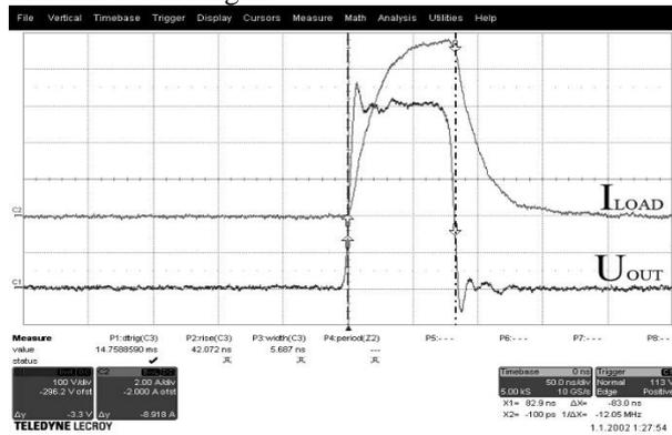
Figure 6. An 80 ns 500 V pulse  $U_{OUT}$  generated on the output of the test board. Current through a 50  $\Omega$  load resistor is demonstrated. (50 ns/div, 100 V/div and 2 A/div)
