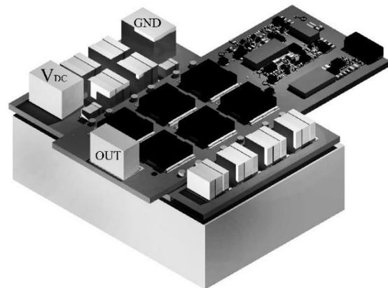
Figure 4. PCB board with marked DC link voltage  $V_{DC}$ , GND and output OUT
