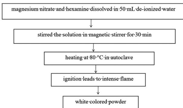
**Figure 2:** Flowchart for the synthesis of NC MgO
