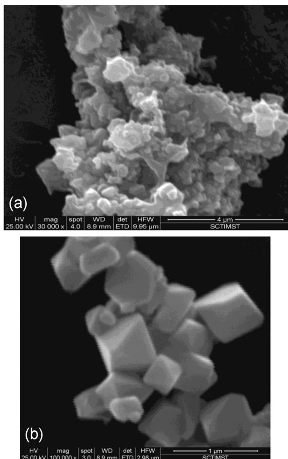
**Figure 3:** SEM images of annealed NC MgO attained by combustion technique: a) mag. 30 000 ×, b) mag. 100 000 ×
