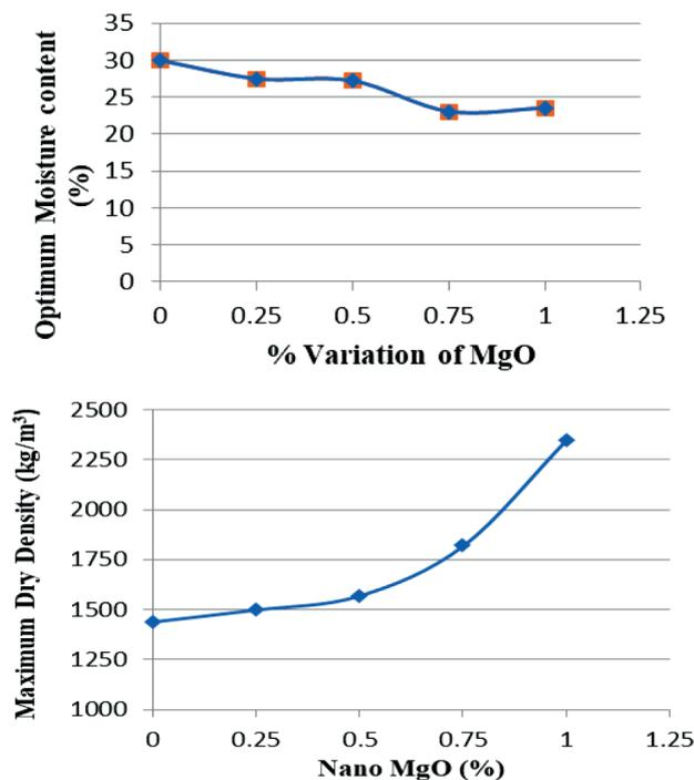
**Figure 5:** Outcomes of compaction study: a) OMC vs MgO, b) MDD vs MgO
