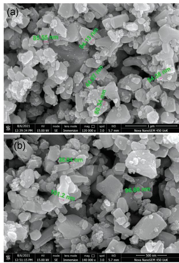
**Figure 4:** FE SEM images of nano ZnO powders: a) mag. 120 000 ×, b) mag. 140 000 ×
