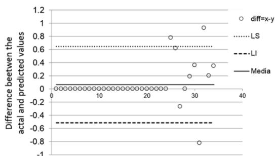
Fig. 8. Bland-Altman plot for ANFIS model of surface roughness
