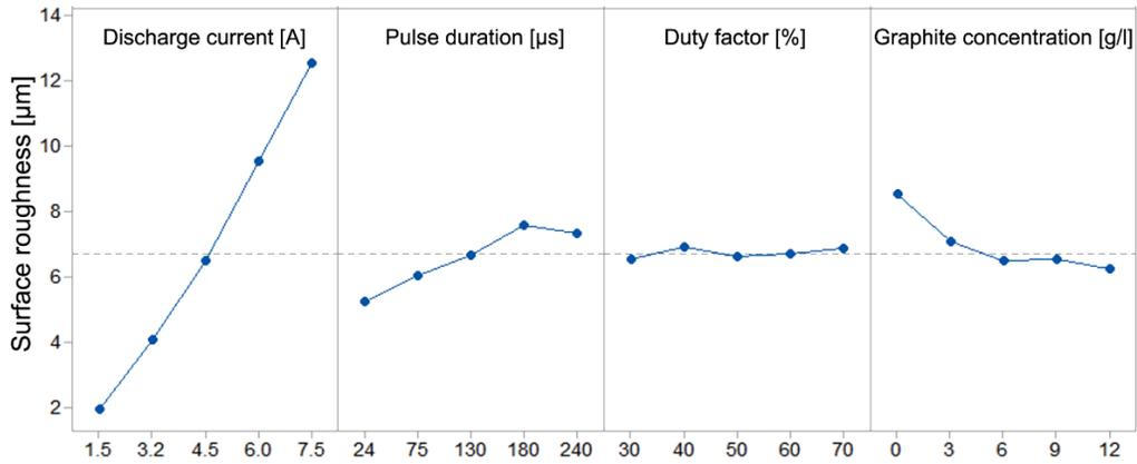
Fig. 11. Main effect plot for surface roughness
