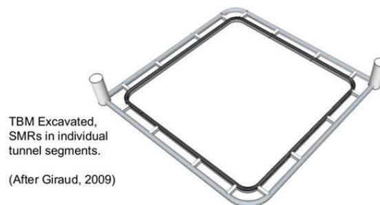
**Figure 10:** Twelve unit installation<sup>[10]</sup>.
