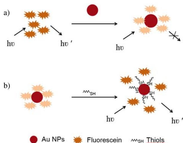
**Scheme 1:** Schematic representations of fluorescent probe for thiols detection
