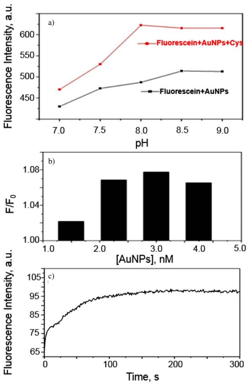
Fig. S1. Effects of pH (a), AuNPs concentration (b), and reaction time (c) on the enhancement of fluorescence.
