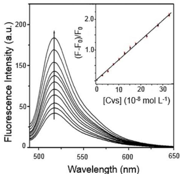
Fig. 4: Fluorescent spectra of fluorescein-AuNPs complex in the presence of different concentrations of cysteine. Inset is the calibration curve of  $(F-F_0)/F_0$  versus the concentration of cysteine. The concentrations of cysteine (from bottom to top) were: 0, 2.5, 5.0, 7.5, 10.0, 12.5, 15.0, 17.5, 22.5, 27.5, 32.5  $\times 10^{-8}$  mol L<sup>-1</sup>
