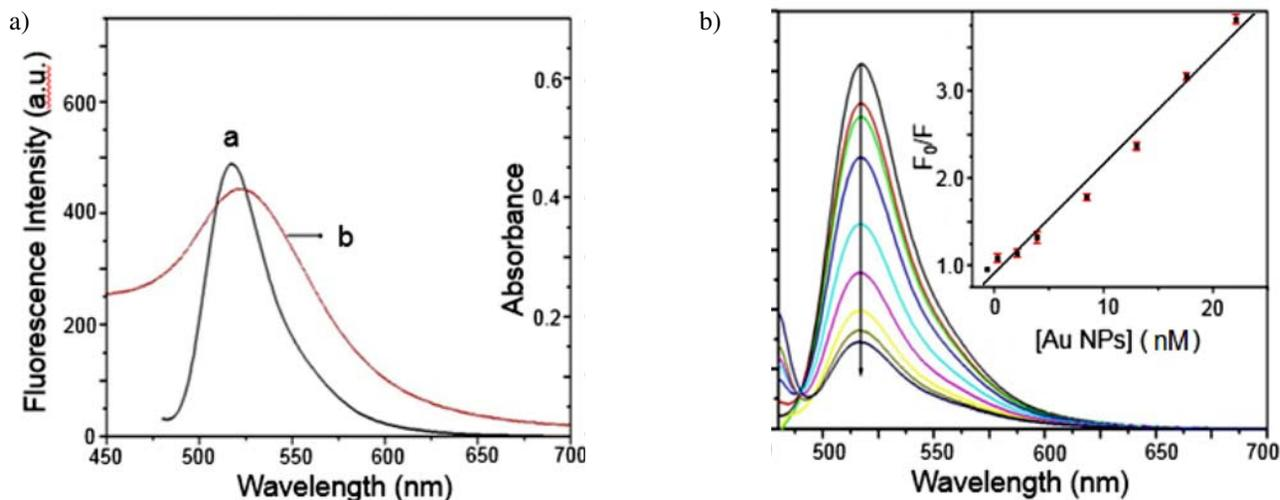
Fig. 2: a) Emission spectrum of fluorescein (curve a) and absorption spectrum of AuNPs (curve b); b) Fluorescent spectra of fluorescein upon addition of AuNPs with various concentrations. The inset shows the relationship between  $F_0/F$  versus  $[\text{AuNPs}]$ . Fluorescein:  $1.5 \times 10^{-7}$  mol L<sup>-1</sup>; AuNPs (from top to bottom): 0.0, 0.88, 2.6, 4.2, 8.5, 13, 17, 21, 23  $\times 10^{-10}$  mol L<sup>-1</sup>
