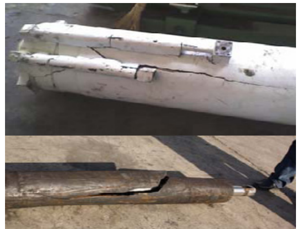
Fig. 1. The damaged hydraulic cylinders
