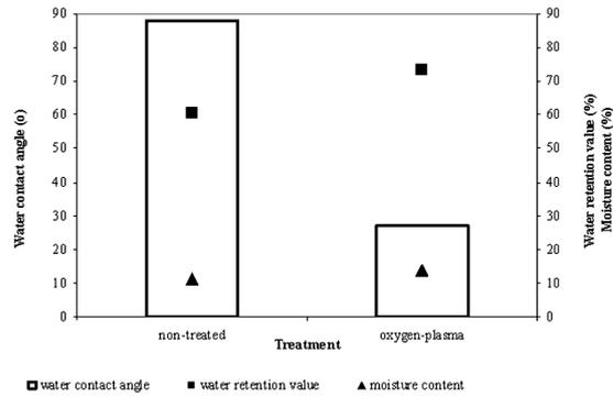
**Figure 2:** Hydrophilic/hydrophobic properties of a non-treated and oxygen plasma treated regenerated non-woven cellulose sample
