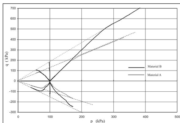
Figure 9. S\_BRICK predictions of drained triaxial shearing taken at different directions at normally consolidated state for the materials A and B.
