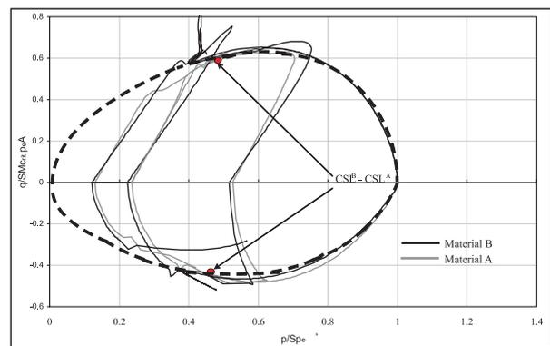
**Figure 13.** State boundary surface in the  $q/SM^{crit}p_e^A - p/Sp_e^A$  plot.
