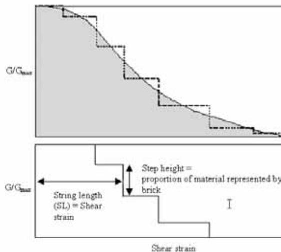
Figure 4. Discretization of the *S-shaped curve* by Simpson [2].
