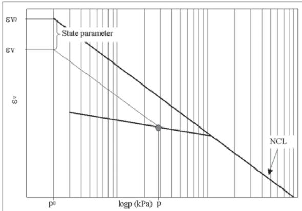
**Figure 5.** The concept of the state parameter as modeled in BRICK.
