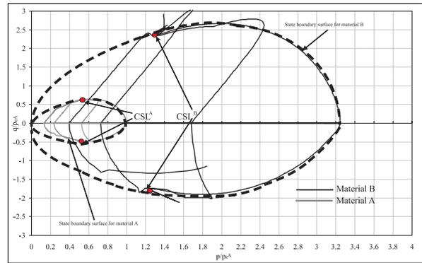
**Figure 12.** State boundary surfaces in the  $q/p_e^A - p/p_e^A$  plot.
