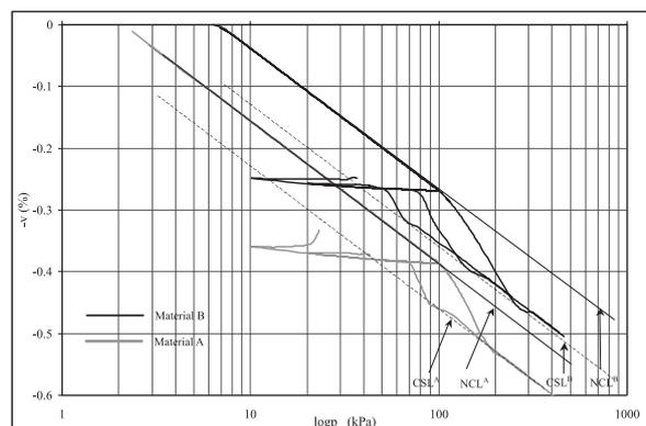
Figure 8. S\_BRICK predictions of normal compression and swelling with drained triaxial shearing taken at different states for the materials A and B.
