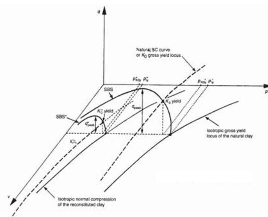
Figure 3. Theoretical framework for structured and reconstituted material in the q-p-v space by Cotecchia & Chandler [1].
