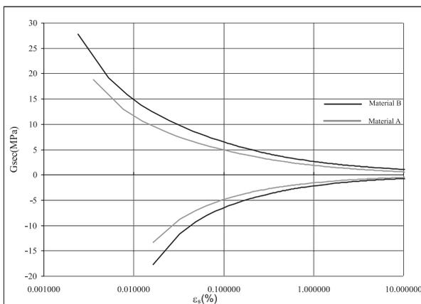
**Figure 11.** S\_BRICK prediction of shear stiffness response in triaxial compression and extension shearing tests.
