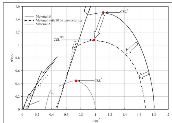
Figure 16. Destructuring in shearing in the  $q/p_e^a - p/p_e^a$  plot.
