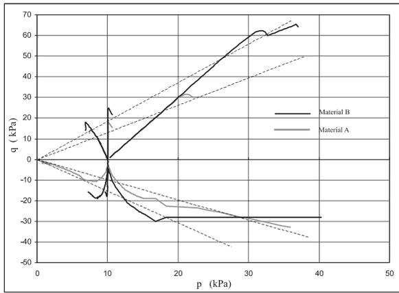
**Figure 10.** S\_BRICK predictions of drained triaxial shearing taken at different directions at heavily overconsolidated state (OCR=10) for the materials A and B.
