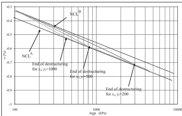
Figure 14. Different rates of destructuring at normal compression.
