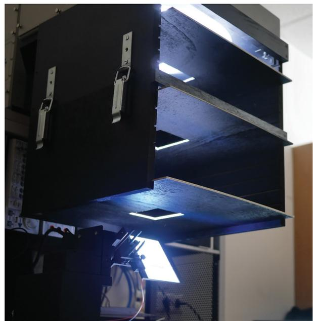
**Figure 7:** A cascade system of masks that limit the light beam in order to minimize the stray light errors.
