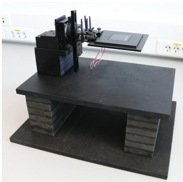
**Figure 1:** The rotary stage mounted onto the supporting construction. A DUT is mounted into a Plexiglas adapter which is then attached to the rotary stage through the two-screw optical filter holder.
