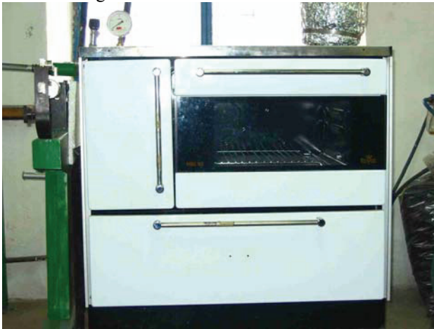
Figure 2: Combined cooker-boiler MBS 90KV on the test rig
