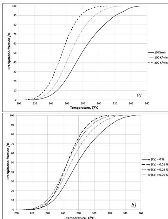
**Figure 6:** Fraction of Al<sub>2</sub>Cu precipitates with respect to the temperature in the AlSi9Cu3 alloy at various cooling rates (a) and at various concentrations of Ce (b)
