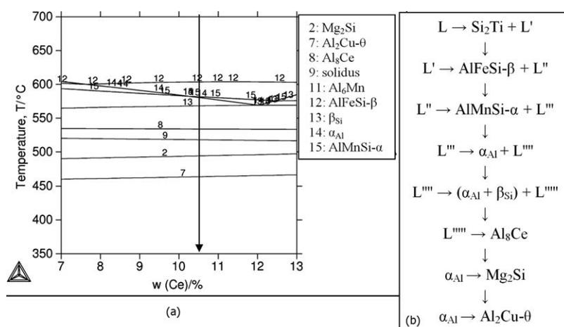
**Figure 1:** Equilibrium phase diagram (a) and schematic representation of equilibrium solidification of AISi9Cu3 alloy with  $w = 0.02\text{ } \%$  Ce
